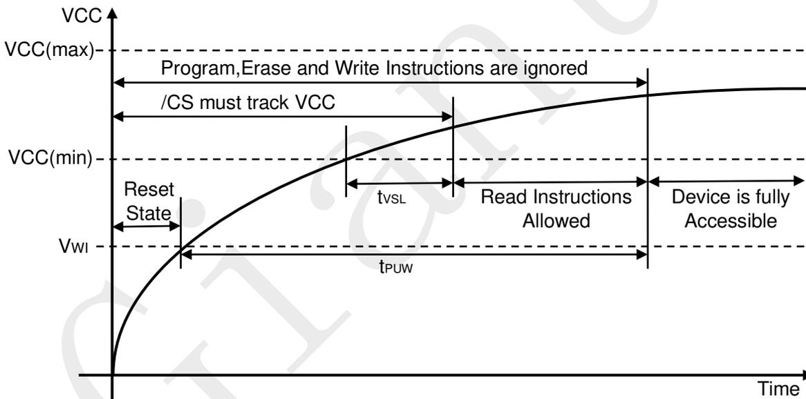
Power-up Timing and Voltage Levels
