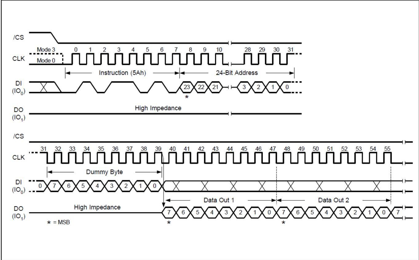
Figure 30. Read SFDP Register Instruction Sequence Diagram(SPI mode only)
