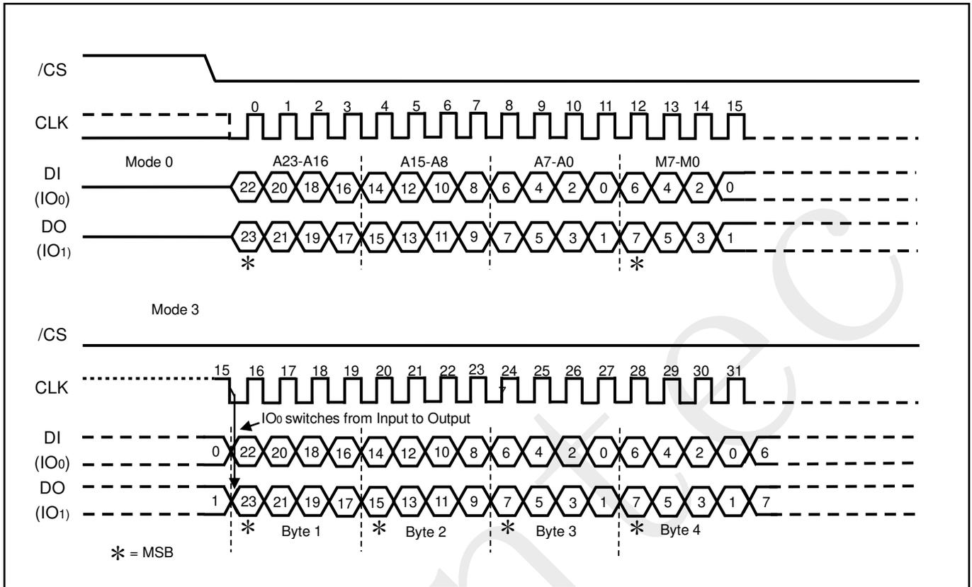
Figure10a. Dual/O Fast Read Sequence Diagram (M5-4= (1, 0))
