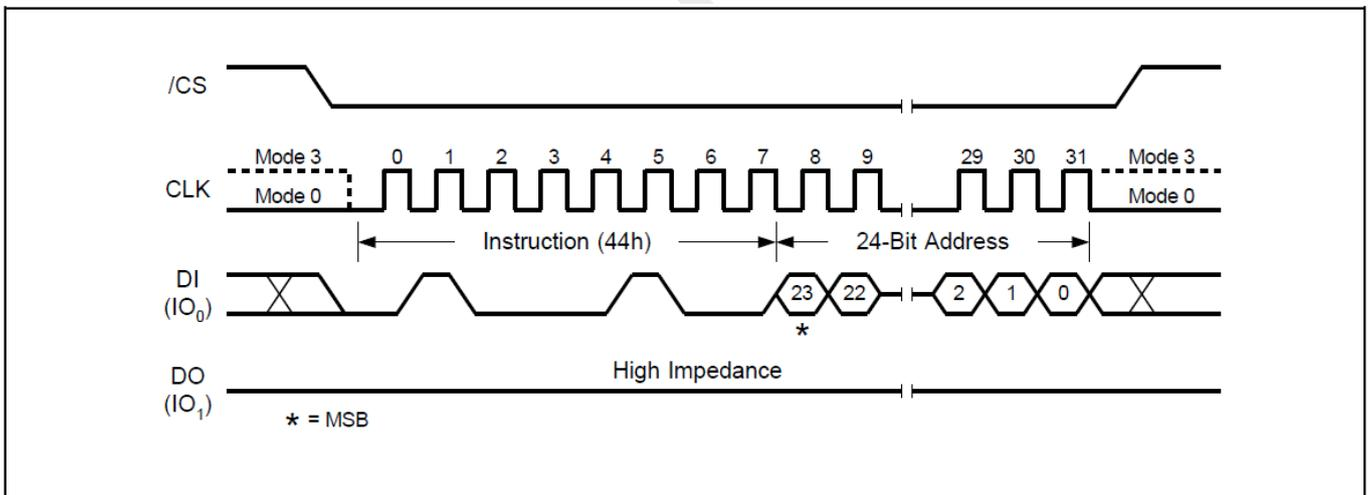
Figure 31. Erase Security Registers Instruction (SPI Mode only)
