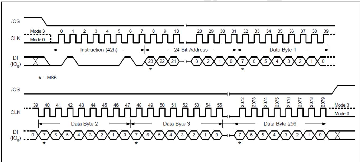
Figure 32. Program Security Registers Instruction (SPI Mode only)
