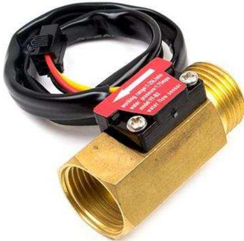
It consists of a copper body, a water rotor, and a hall-effect sensor. When water flows through the rotor, rotor rolls. Its speed changes with different rate of flow. The hall-effect sensor outputs the corresponding pulse signal.
