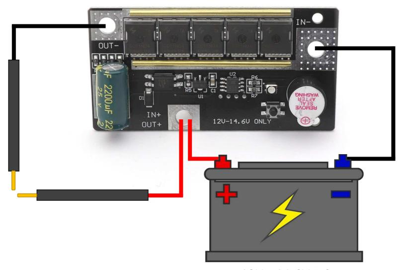
12V...14.6V DC min. 30Ah - max. 45Ah lead-acid battery
