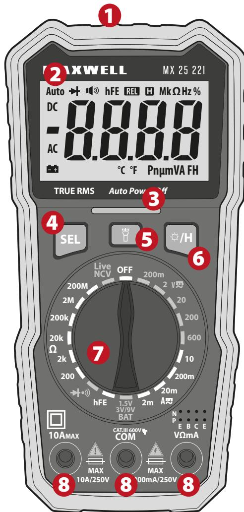
**① NCV Non-Contact-Voltage detection/ Work light**
