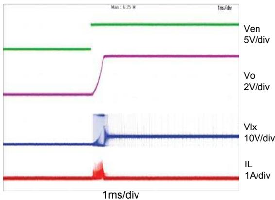
**Start-up Through Enable with  $I_{OUT} = 1\text{ A}$  Resistive Load**
