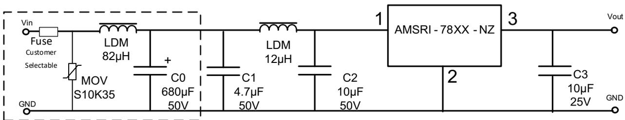
**NOTE:** This part is not designed for parallel operation, only input parallel supply to achieve positive and negative output
