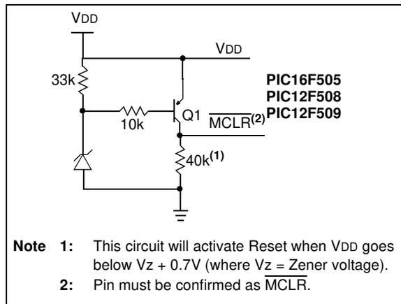
**FIGURE 7-14: BROWN-OUT PROTECTION CIRCUIT 2**
