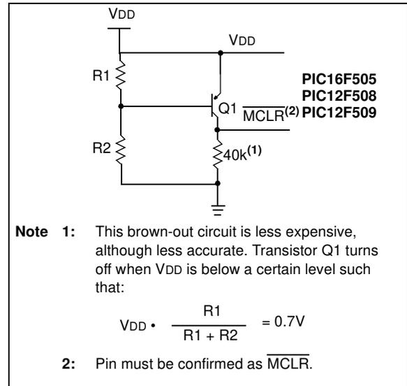
**FIGURE 7-15: BROWN-OUT PROTECTION CIRCUIT 3**
