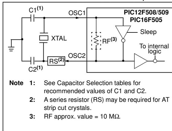
**FIGURE 7-2: EXTERNAL CLOCK INPUT OPERATION (HS, XT OR LP OSC CONFIGURATION)**
