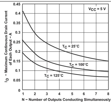
Figure 6. Maximum Continuous Drain Current of Each Output vs Number of Outputs Conducting Simultaneously
