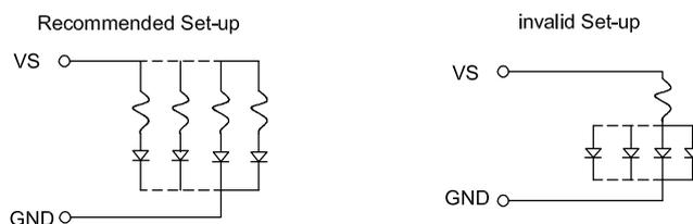
3. The driving circuit should be designed to protect the LED against reverse voltages and transient voltage spikes when the circuit is powered up or shut down.
