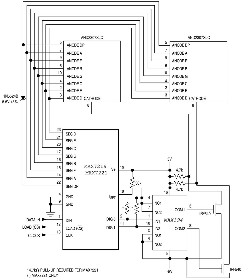
Figure 2. MAX7219/MAX7221 Driving 2.3-Inch Displays
