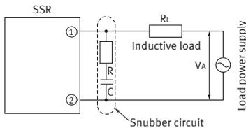
If there is no resistance R (the resistance R controls the discharge current from condenser C), at turn-on of the SSR, there will be a sharp rise in dv/dt and the high peak value discharge current will begin to flow.
