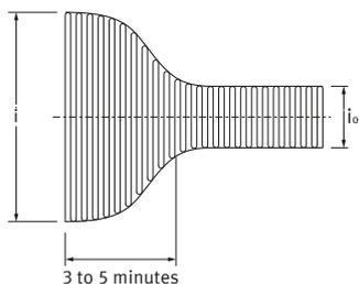
The discharge tube, transformer, choke coil, capacitor, etc., are combined in common discharge lamp circuits. Note that the inrush current may be 20 to 40 times, especially if the power supply impedance is low in the high power factor type.
