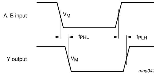
For 74HC1G86:  $V_M = 0.5 \times V_{CC}$ ;  $V_I = \text{GND to } V_{CC}$ .
