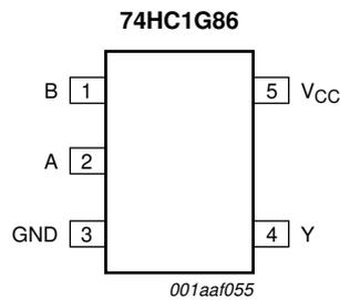
Fig 4. Pin configuration
