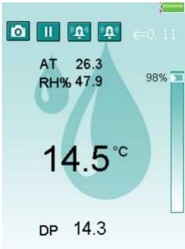
In the Dew Point mode the percentage bargraph indicates how close the IR temperature is to the Dew Point temperature. At 100%, the two values are identical.
