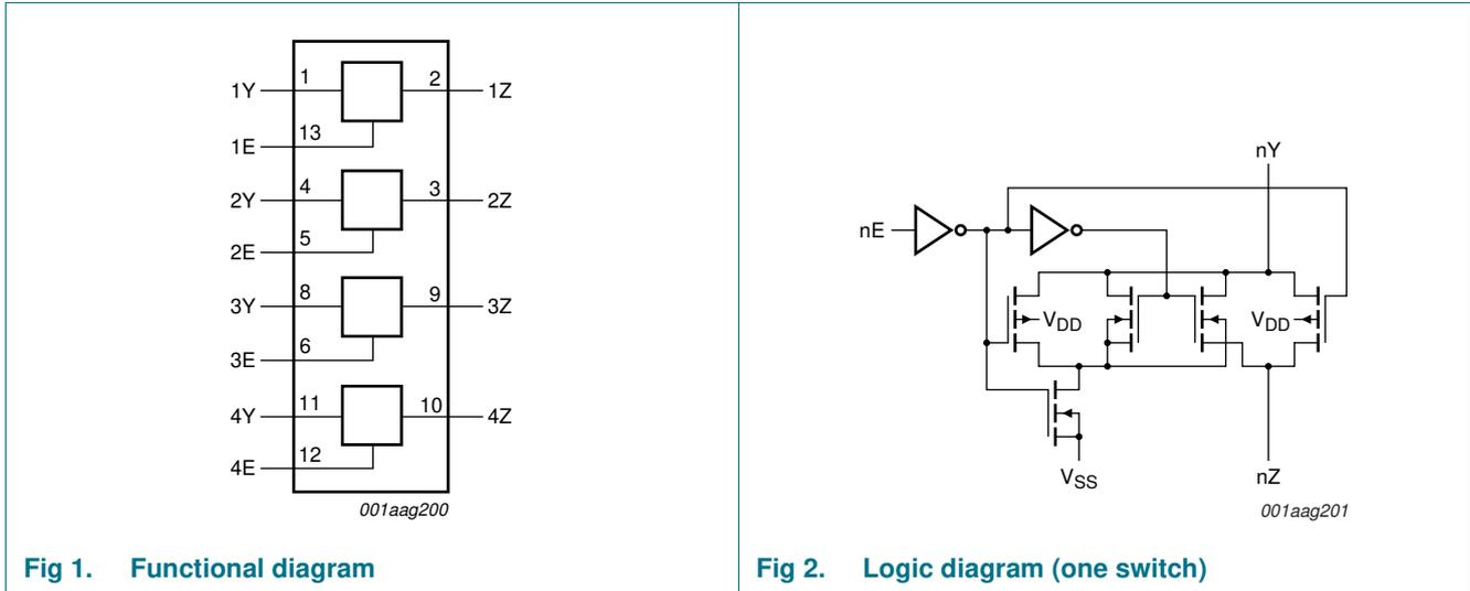
Fig 1. Functional diagram
