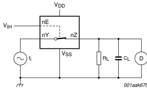
Fig 10. Test circuit for measuring total harmonic distortion
