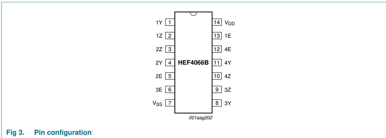
Fig 3. Pin configuration
