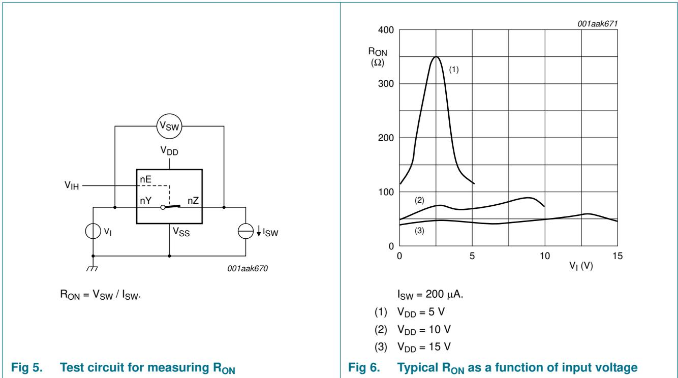
Fig 5. Test circuit for measuring  $R_{ON}$
