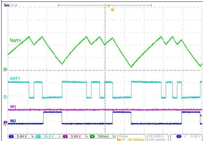
Figure 12. Current Regulation With VREF = 2 V and 150 mΩ
