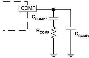
**C<sub>COMP2</sub> is needed only for high ESR output capacitor**
