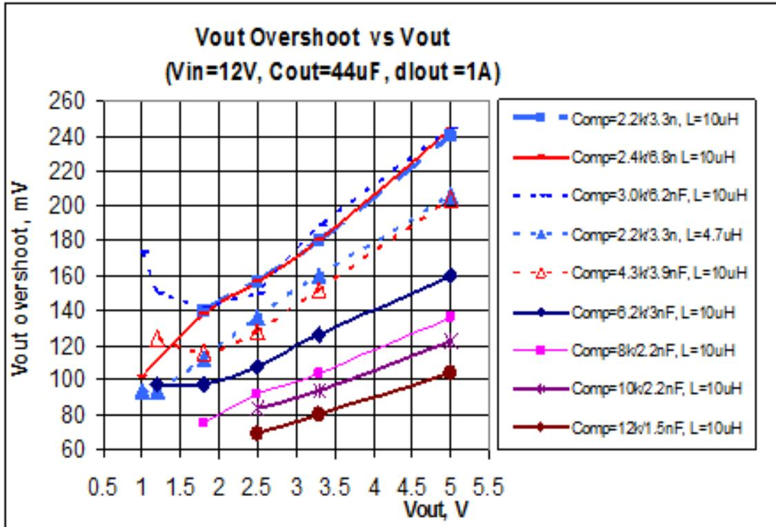
Figure 3. Load Transient Testing VS Compensation Value
