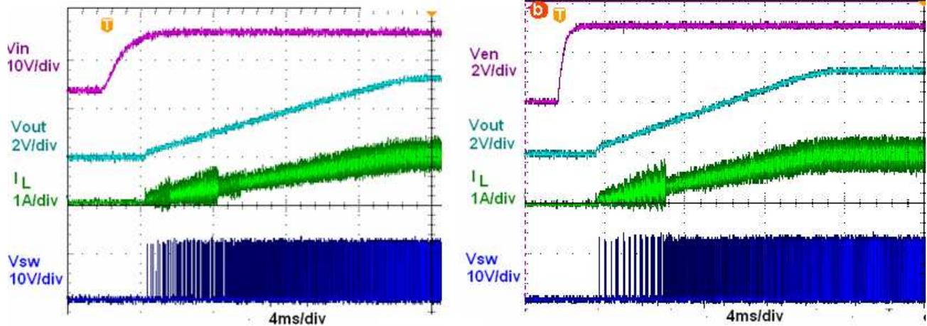
**Short Circuit Protection  $V_{in}=12V$**
