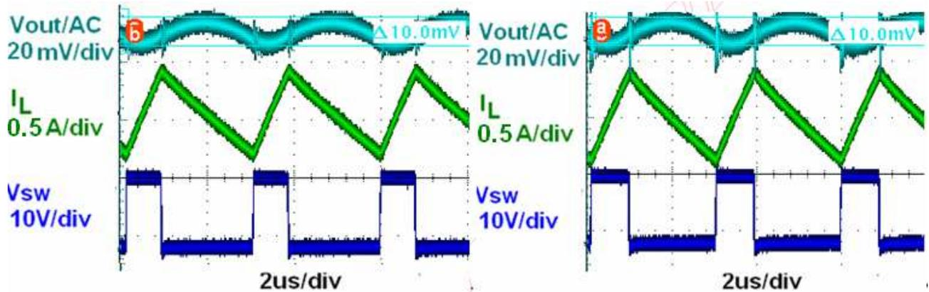
**Startup  $V_{in}=12V$ ,  $V_{out}=3.3V$ ,  $I_{out}=1A$
