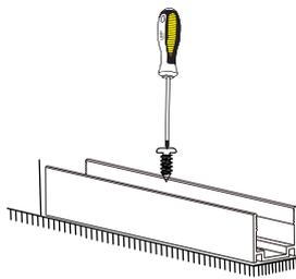
Overall dimension of aluminum profile: L1000\*W13\*H5.8mm
