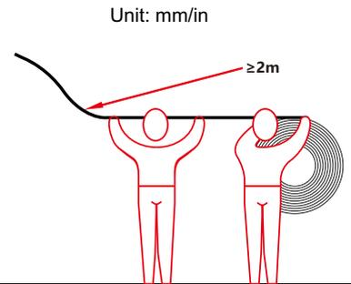
When the length of neon light strip is more than 2 meters, two people are required to install it together.
