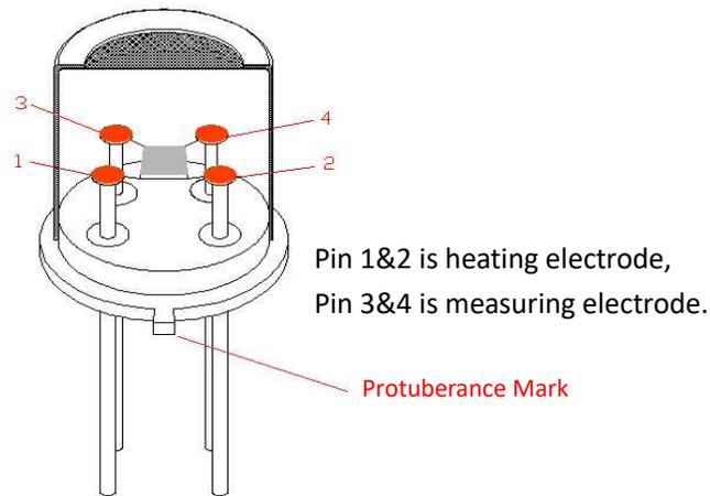
**Fig8.Pin Schematic Diagram**
