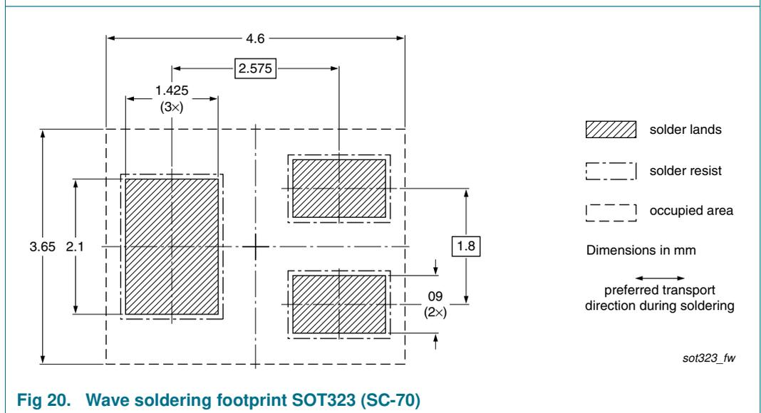
**Fig 20. Wave soldering footprint SOT323 (SC-70)**
