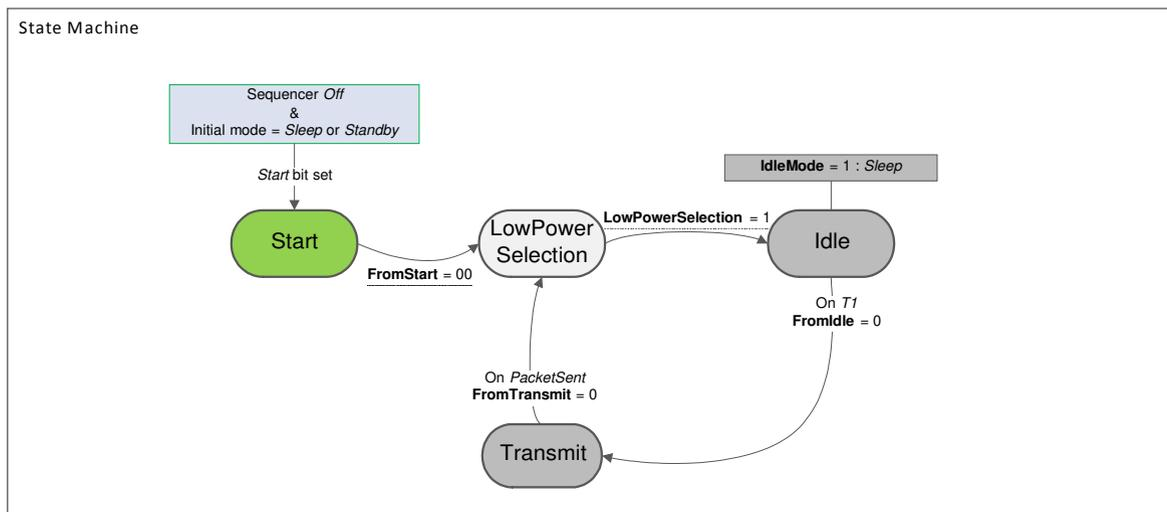
Figure 53. Beacon Mode State Machine
