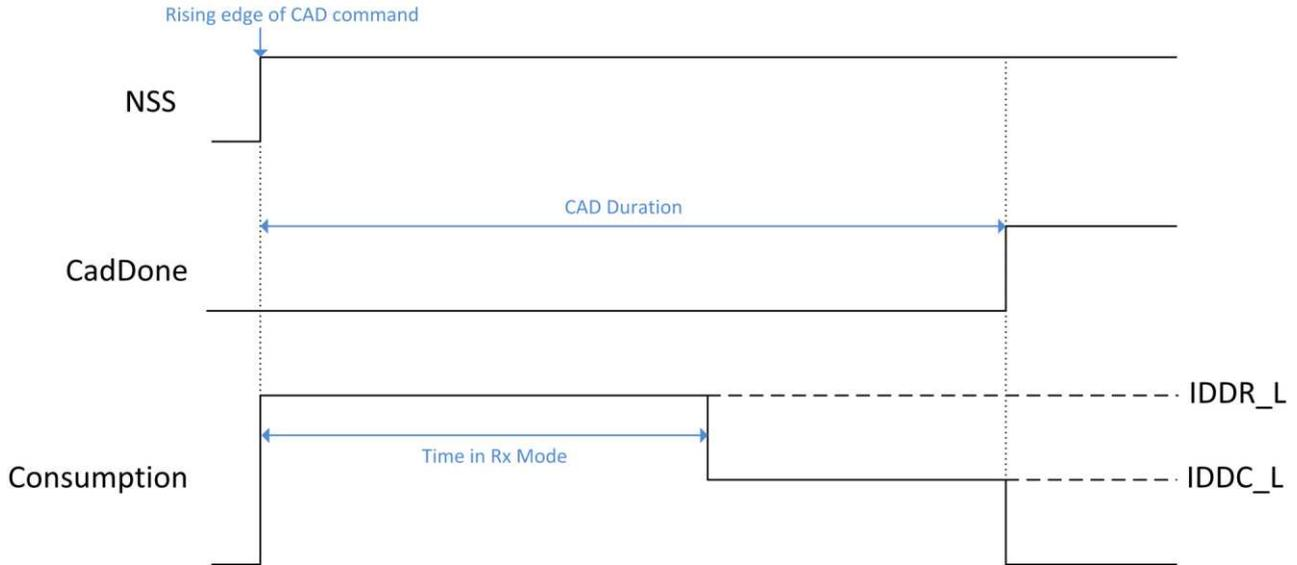
Figure 12. Consumption Profile of the LoRa CAD Process
