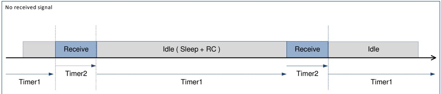
Figure 45. Listen Mode with No Preamble Received
