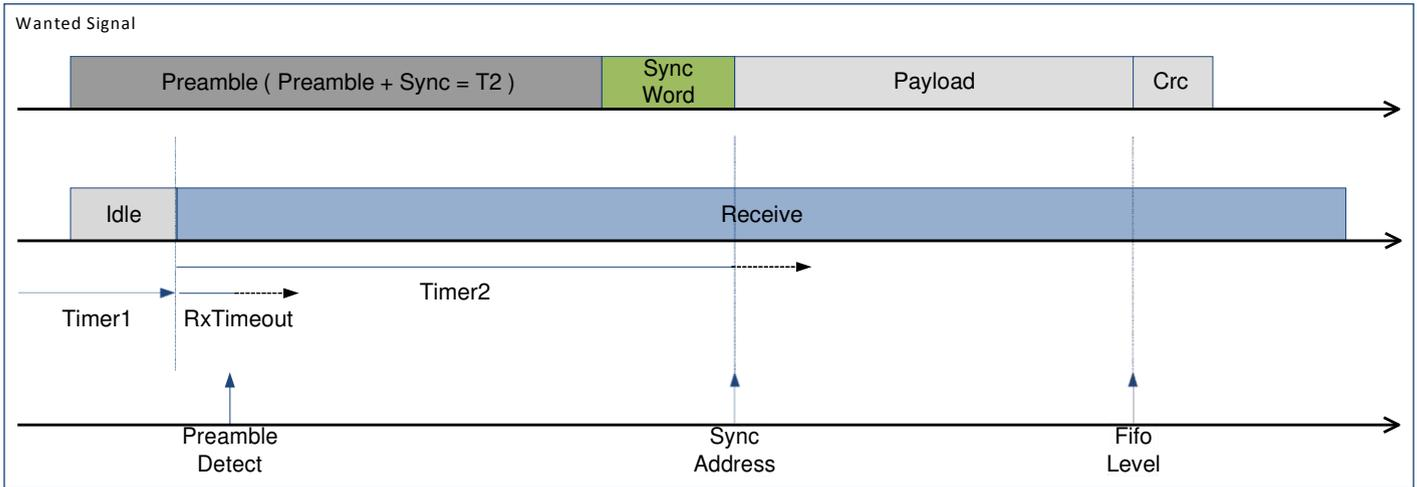
Figure 50. Listen Mode with Preamble Received & Valid SyncAddress
