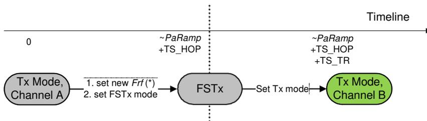
Figure 22. Transmitter Hopping
