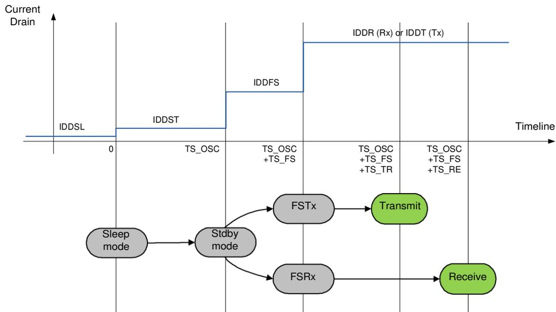
Figure 17. Startup Process
