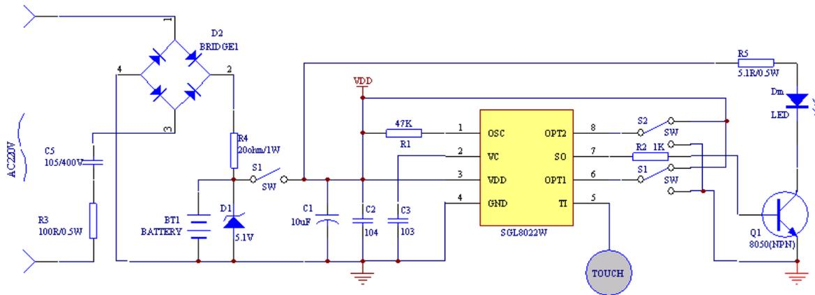
Figure 2. graph of applied circuit with rechargeable battery as the power supply
