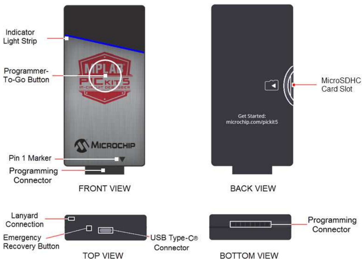
Figure 5-1. MPLAB® PICKit™ 5 In-Circuit Debugger Diagram
