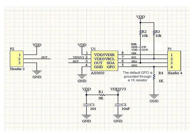
This module is mainly placed behind the stepper motor to obtain the rotation angle of the stepper motor
