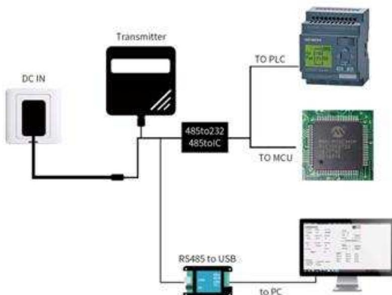
This product can also be used by multiple sensors combined in a 485 bus. In theory, one bus can connect more than 16 485 sensors. If more 485 sensors are needed, more 485 devices can be expanded using 485 repeaters. The other end is connected to the PLC、with 485 interface chip through 485 interface chip, or can be connected to the computer by using USB to 485, the sensor configuration tools provided by our company to configure and test.
