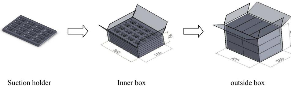
Packaging of snap-in and lead types supercapacitor:
