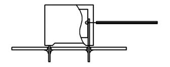
Temperature monitored inside the capacitor.
