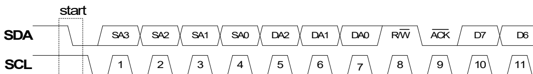
Figure 13-5. Addressing an I2C Peripheral
