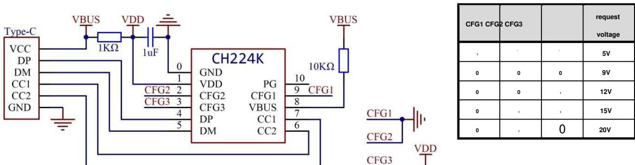
6.3. CH224K uses Type-C male port, only uses PD protocol and E-Mark simulation function (the resistor configuration NC in the figure is 20v)
