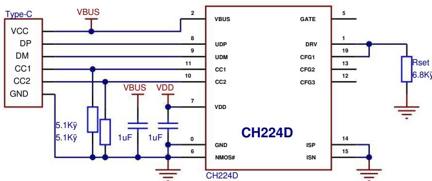
6.2. CH224K uses Type-C female port, the level configuration is 5/9/12/15/20V (the level configuration in the figure is 12v)
