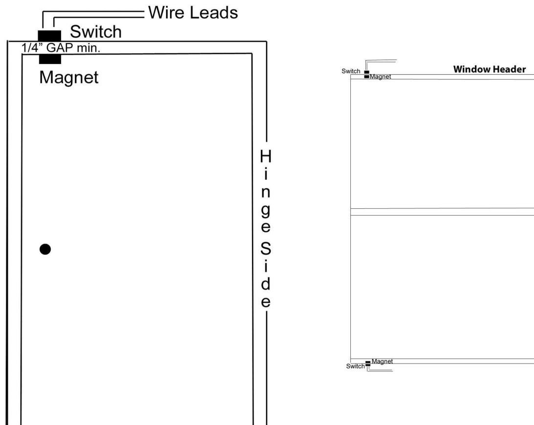
Surface mount switch at top or side (NOT on hinge side) of door or hinged window frame
