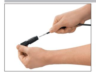
▶ Insert the crimped contact evenly into the housing until the contact has reached its end position and a "click" can be heard.
