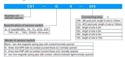
Note: The quick joint that is attached at the end of wire is three-needle-male joint-linear-rotary screw
