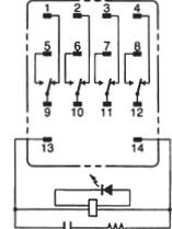
(The coil has no polarity.)
