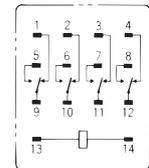
(The coil has no polarity.)
