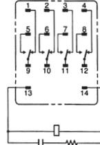
(The coil has no polarity.)
