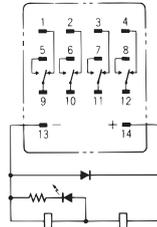
(Check the coil polarity when wiring and wire all connections correctly.)
