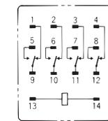
(The coil has no polarity.)
