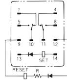
**Note:** R is a resistor for ampere-turn correction. This resistor is built-in to 50-VAC and higher models. (The coil has no polarity.)
