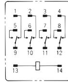
(The coil has no polarity.)
