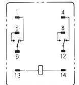
(The coil has no polarity.)
