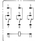
(The coil has no polarity.)
