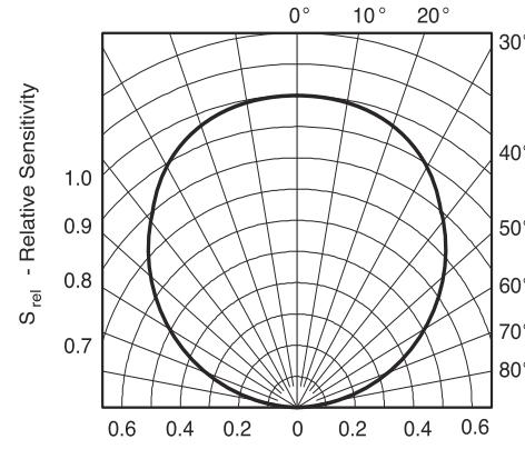
Figure 3. Relative Radiant Sensitivity vs. Angular Displacement
