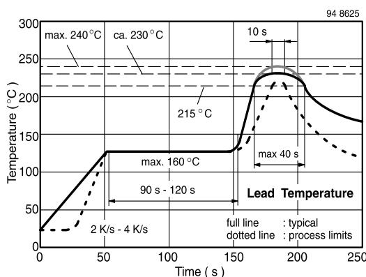
Figure 5. Lead Tin (SnPb) Reflow Solder Profile
