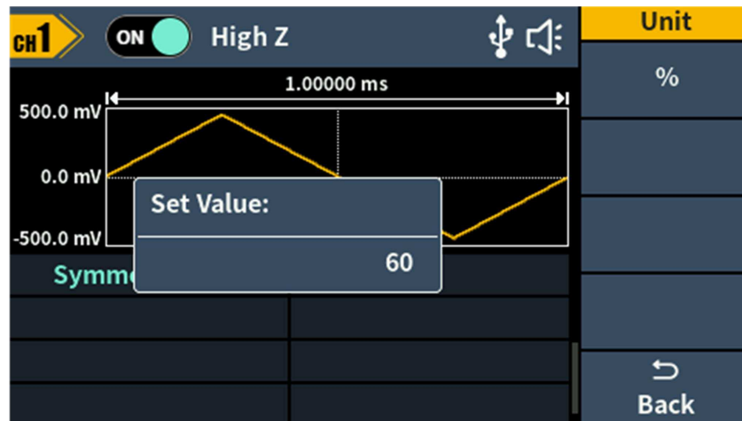
Figure 5- 6: Set the symmetry of ramp wave
