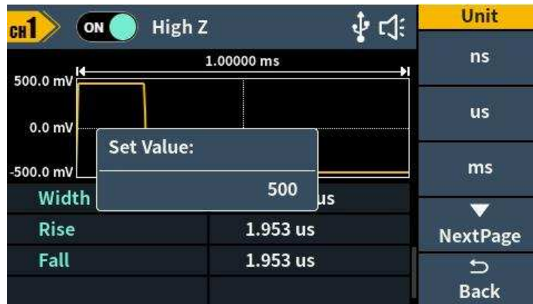
Figure 5-8: Set the pulse width
