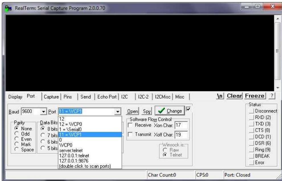
Figure 8: Realterm Port Settings for FTDI Device.
