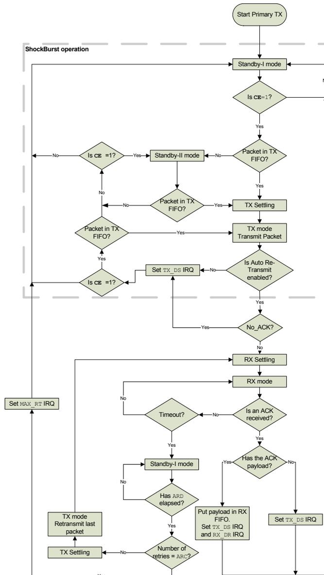
Figure 8. PTX operations in Enhanced ShockBurst™
