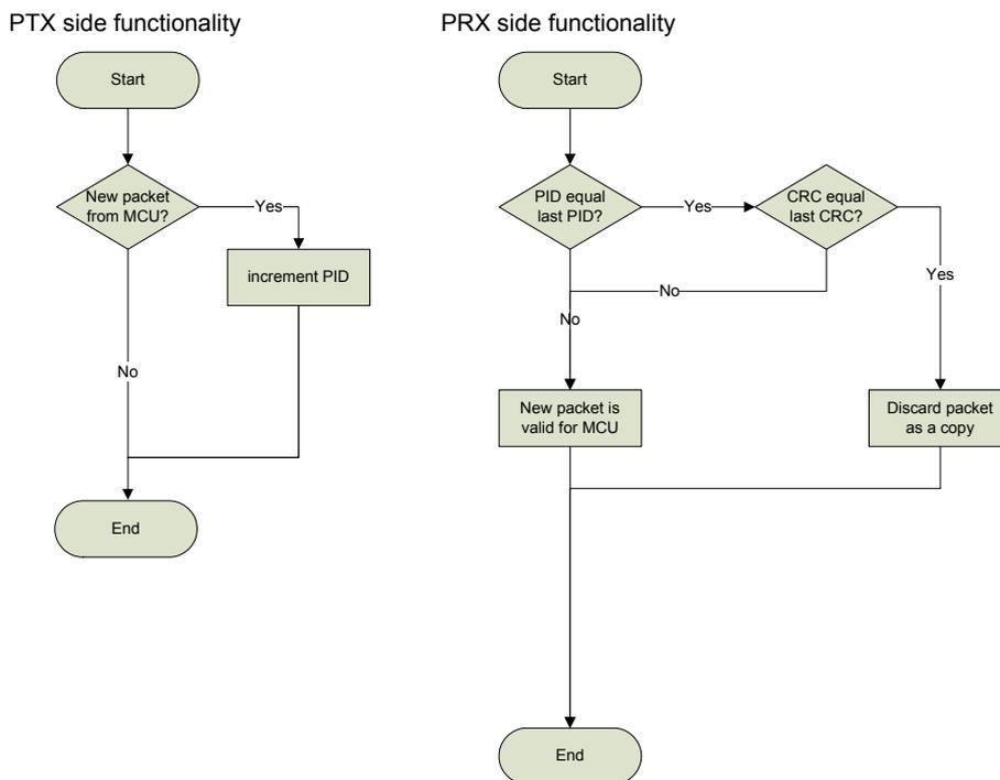
Figure 6. PID generation/detection
