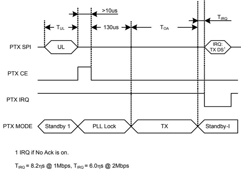
Figure 13. Transmitting one packet with **NO\_ACK** on
