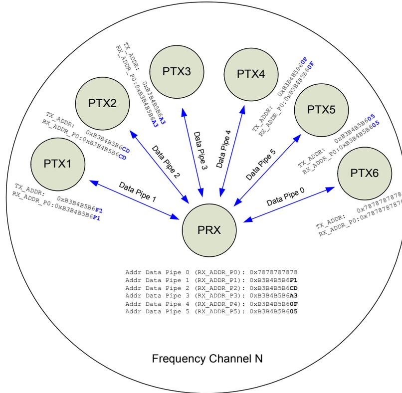
Figure 12. Example of data pipe addressing in multiciever
