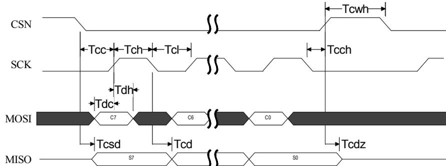
Figure 25. SPI NOP timing diagram
