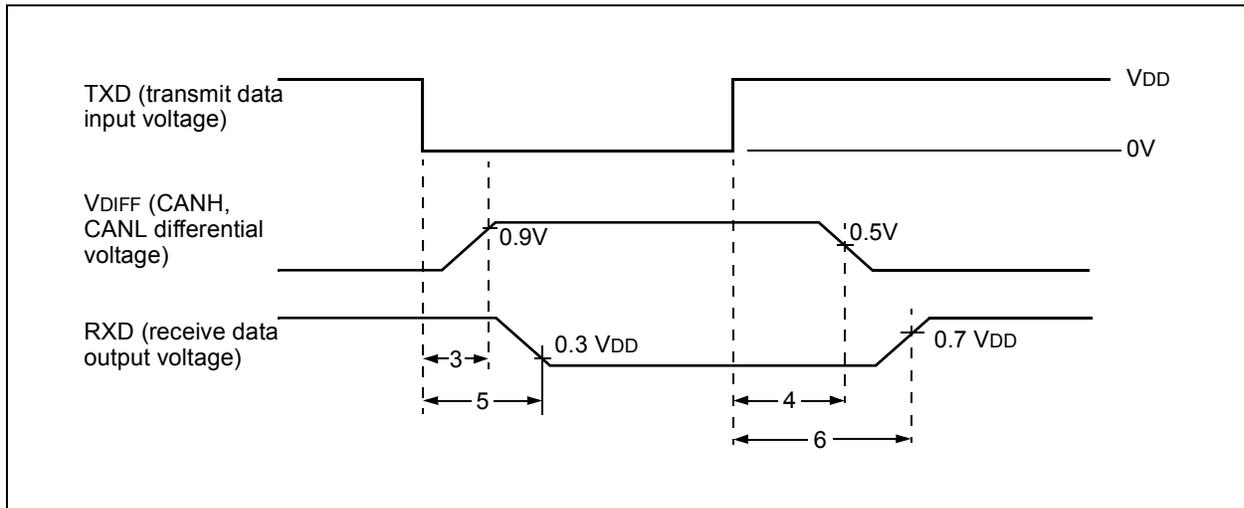
**FIGURE 2-5: TIMING DIAGRAM FOR WAKE-UP FROM STANDBY**
