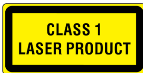
Figure 25. Class 1 laser label
