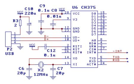
8.3. MCU Read/Write files in USB Flash Disk (File-Level Interface of USB Storage Device)
