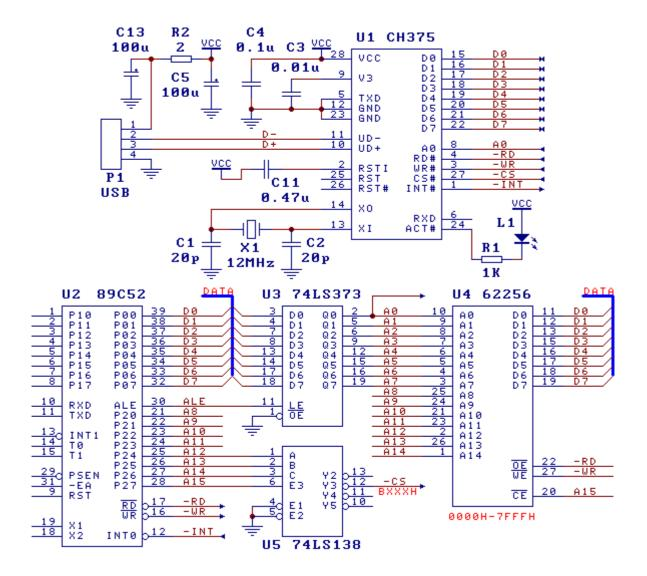
CH375 has a universal passive parallel interface and can be directly connected to a variety of DSP, MCU, etc. In the typical application circuit of MCS-51 series MCU, CH375 can be directly hooked to the system bus of MCU U2 through D7-D0, -RD, -WR, -CS and A0 of the 8-bit passive parallel interface.
