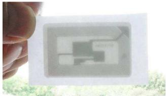
It also supports reading flexible tag. We tested flexible tags of Mifare 1 S50 and Ultralight. The reading distance is up to 5cm.
