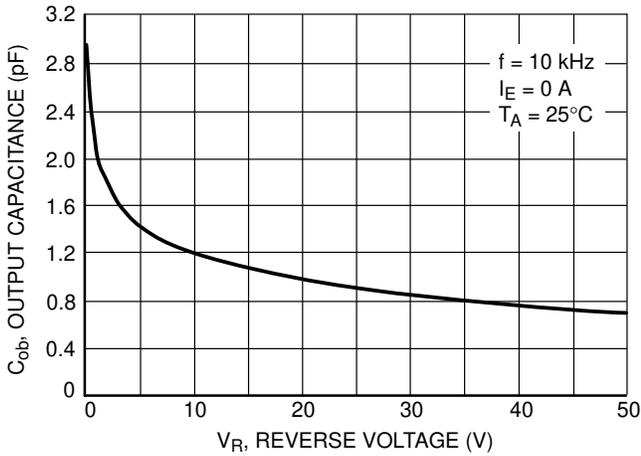
Figure 4. Output Capacitance
