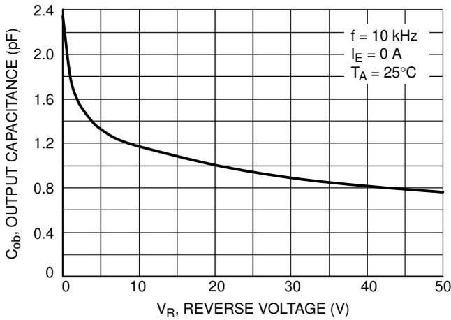
Figure 9. Output Capacitance
