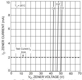
Fig. 4 Typical Zener Breakdown Characteristics
