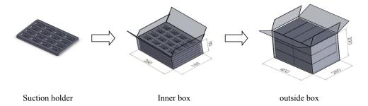
Packaging of Snap-in and Lead Types Supercapacitor:
