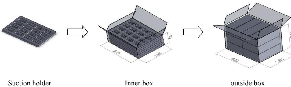
Packaging of Snap-in and Lead Types Supercapacitor:
