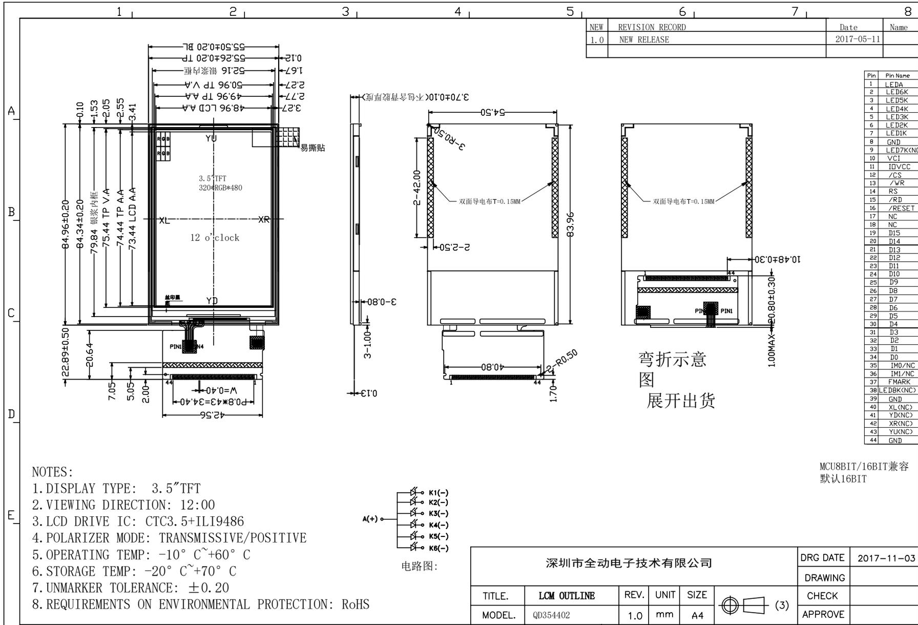
Figure 1: Module specification of the module
