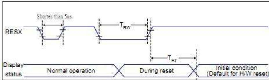
Figure 10 Reset Timing
