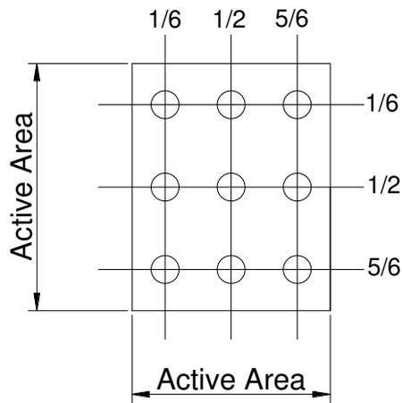
$$U_n = \frac{B_{min}}{B_{max}} \times 100\%$$
