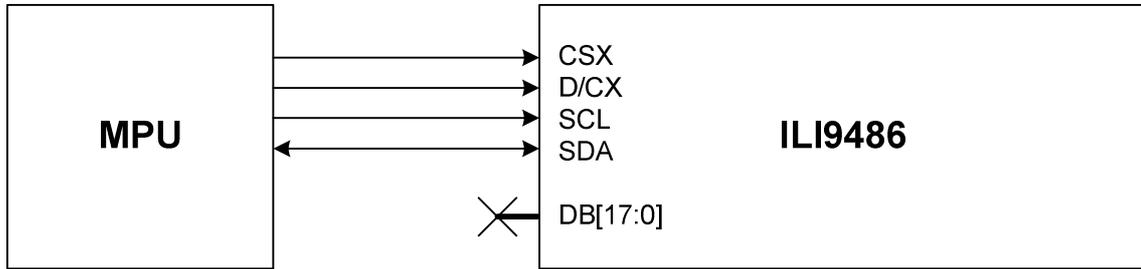
In 4-line serial interface, different display data formats are available for two color depths supported by the LCM listed below.
