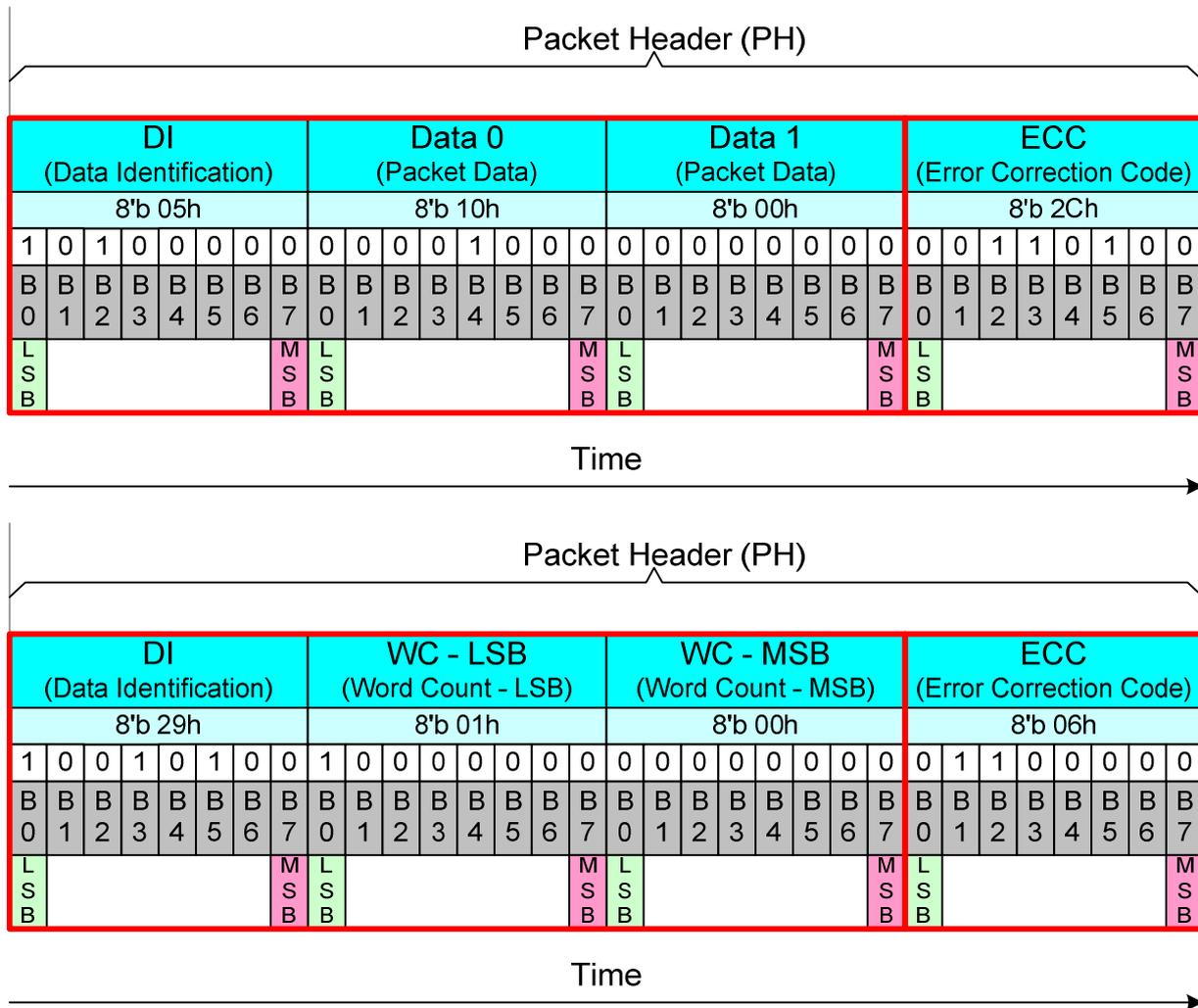
Error Correction Code (ECC) can recognize one error or several errors and makes correction in one bit error case.
