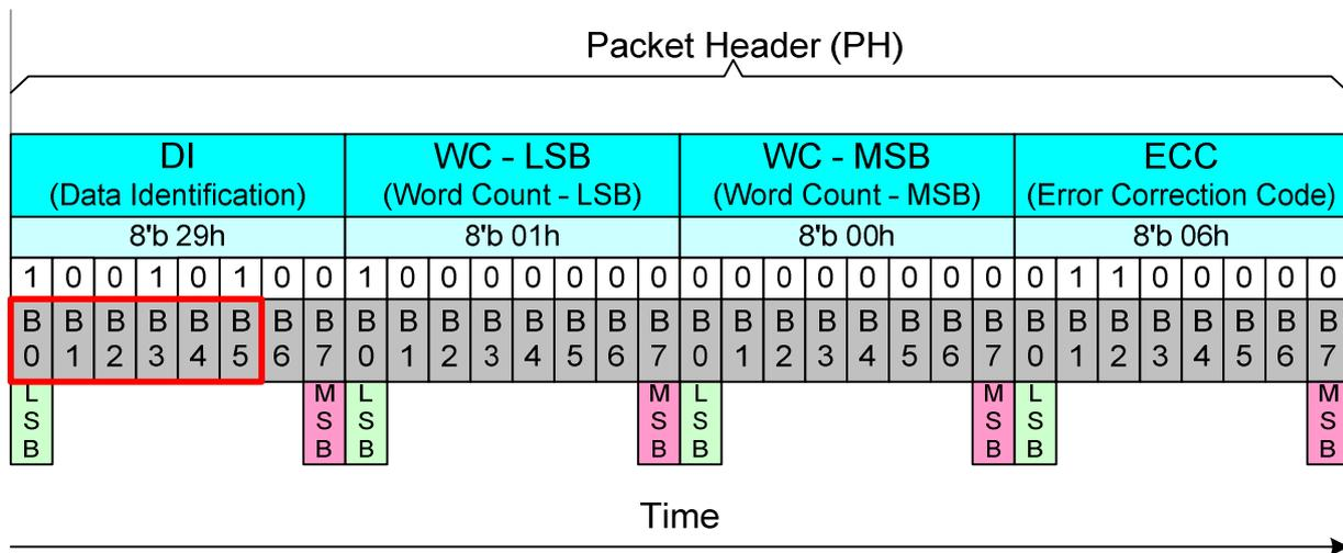
This Data Type (DT) also defines what the used packet is: Short Packet (SPa) or Long Packet (LPa). Data Types (DT) are different from the MCU to the display module (or other devices) and vice versa. These Data Type (DT) are defined on tables below
