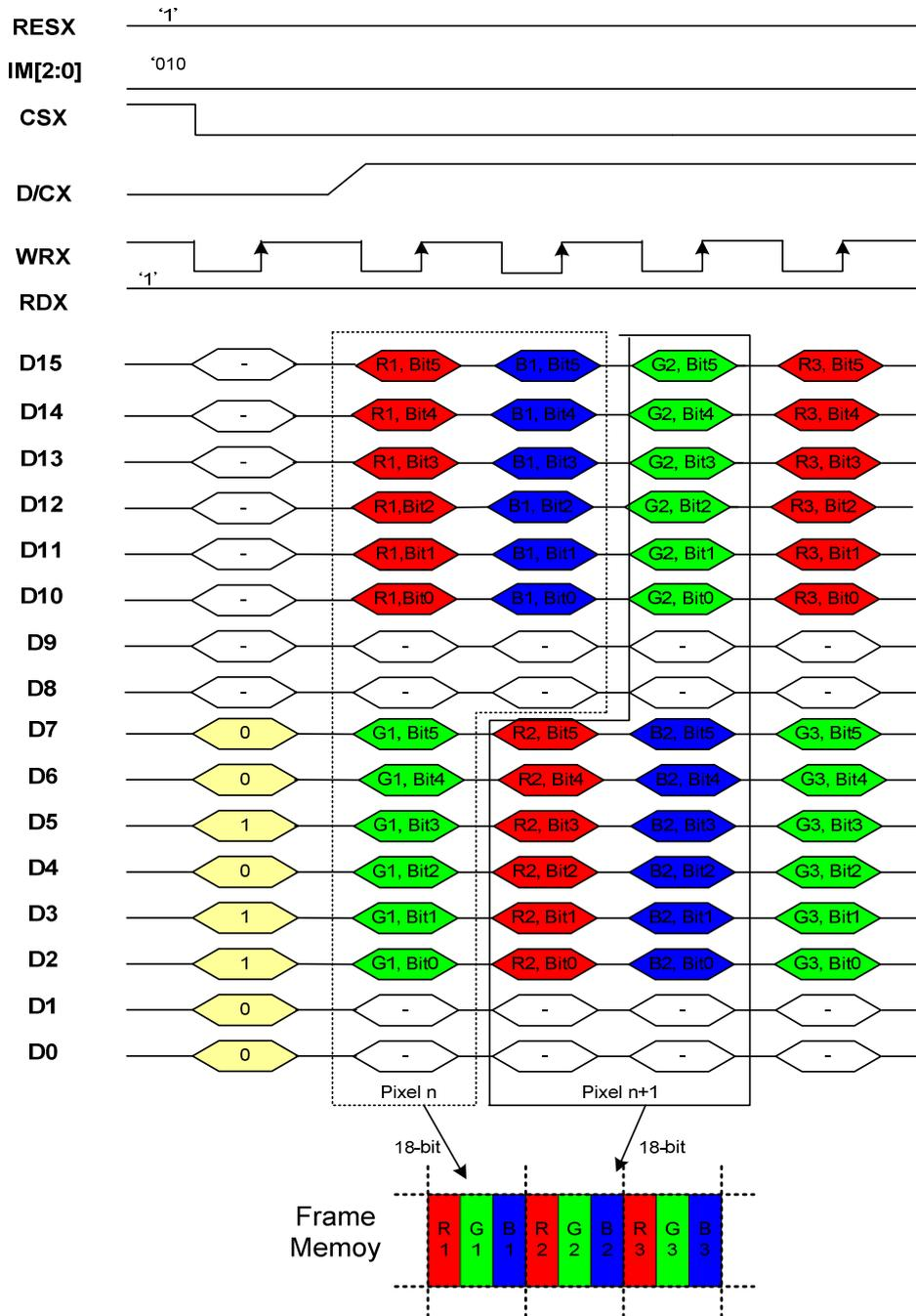
Note 1: The data order is as follows, MSB=D15, LSB=D0 and picture data is MSB=Bit 5, LSB=Bit 0 for Green, Red and Blue data.
