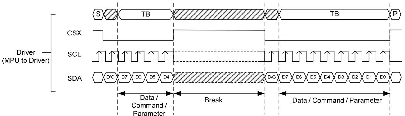
If a two or more parameter command is being sent and a break occurs while sending any parameter before the last one and if the host then sends a new command rather than continue to send the remained parameters that was interrupted, then the parameters that were successfully sent are stored and the parameter where the break occurred is rejected. The interface is ready to receive next byte as shown below.
