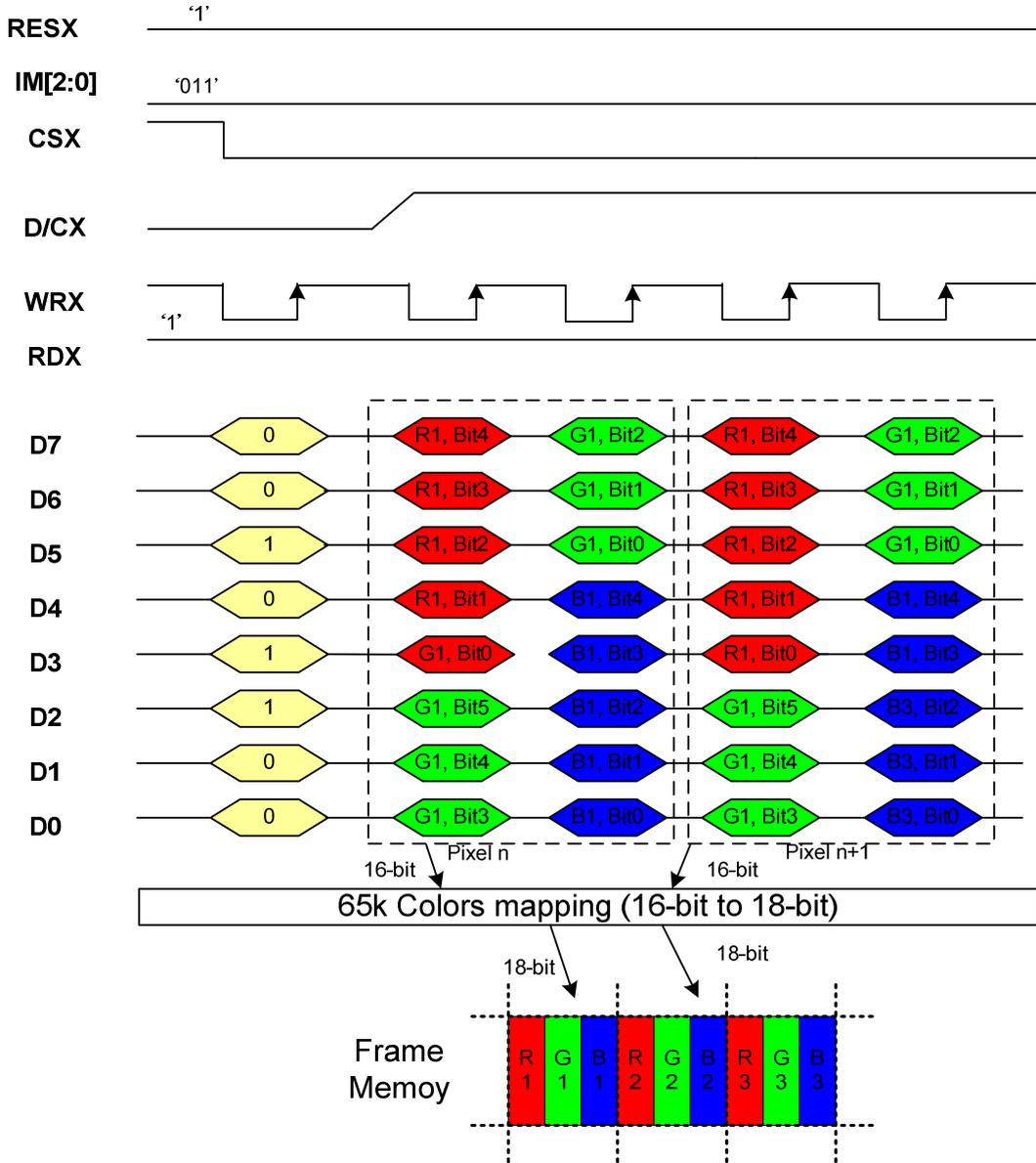
Note 1: The data order is as follows, MSB=D7, LSB=D0 and picture data is MSB=Bit 5, LSB=Bit 0 for Green data and MSB=Bit 4, LSB=Bit0 for Red and Blue data.
