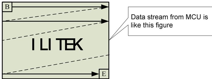
The data is written in the order illustrated above. The Counter which dictates where in the physical memory the data is to be written is controlled by “Memory Data Access Control” Command, Bits B5, B6, and B7 as described below.
