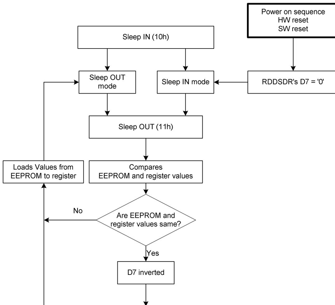
*Note 1: There is not compared and loaded register values, which can be changed by User (User area commands: 00h to AFh and DAh to DDh), by ILI9486.*
