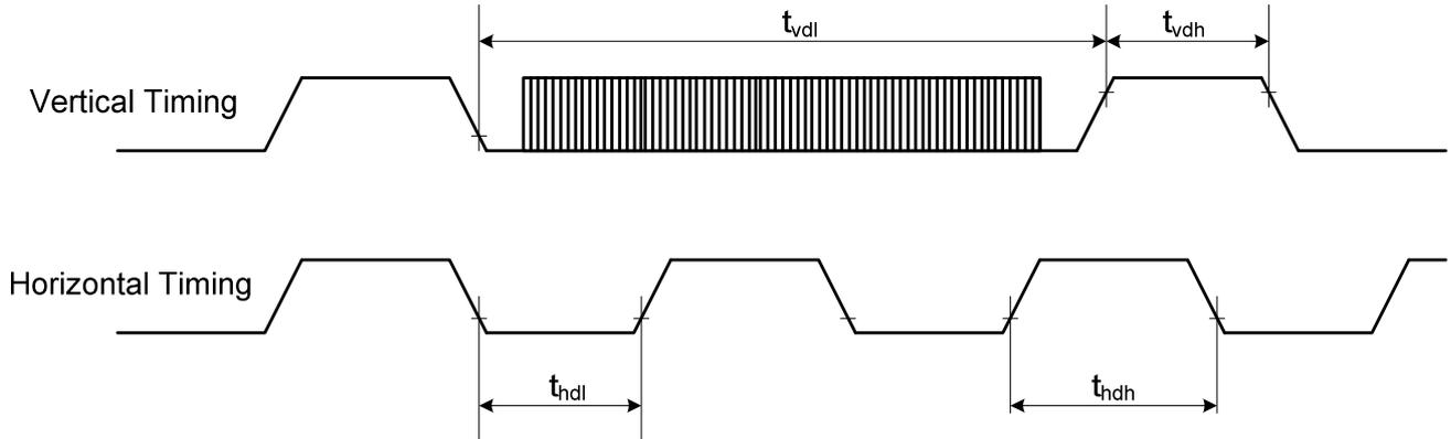
AC characteristics of Tearing Effect Signal (Frame Rate = 60.5Hz)
