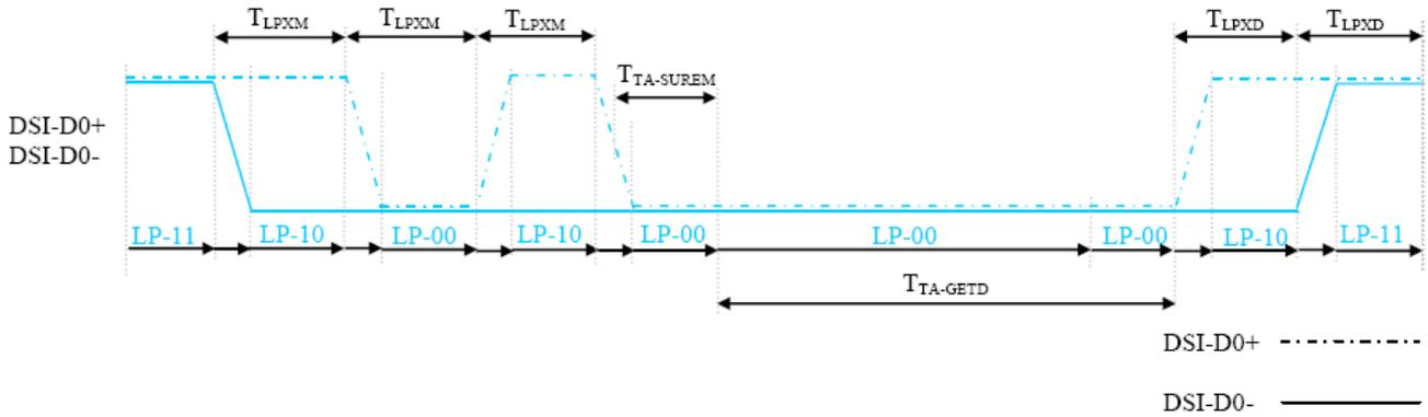
Lower Power Mode and its State Periods are illustrated for reference purposes on the Bus Turnaround (BTA) from ILI9486 to the MCU sequence below.
