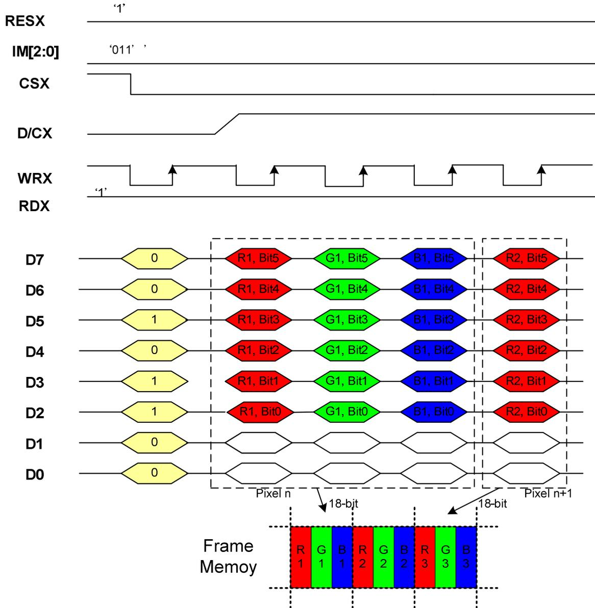
Note 1: The data order is as follows, MSB=D7, LSB=D0 and picture data is MSB=Bit 5, LSB=Bit 0 for Green, Red and Blue data.
