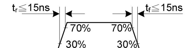
(2) Logic high and low levels are specified as 30% and 70% of IOVCC for input signals.
