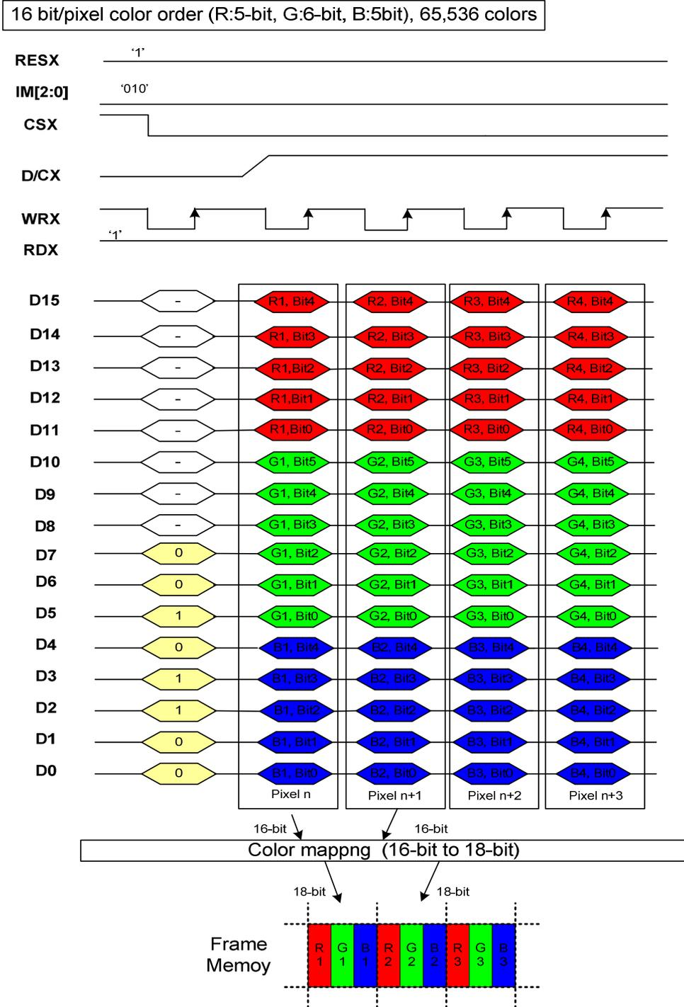
Note 1: The data order is as follows, MSB=D15, LSB=D0 and picture data is MSB=Bit 5, LSB=Bit 0 for Green data and MSB=Bit 4, LSB=Bit0 for Red and Blue data.
