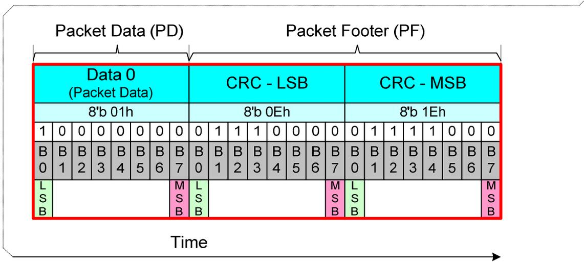
The receiver is calculated own checksum value from received Packet Data (PD). The receiver compares own checksum and the Packet Footer (PF) what the transmitter has sent.
