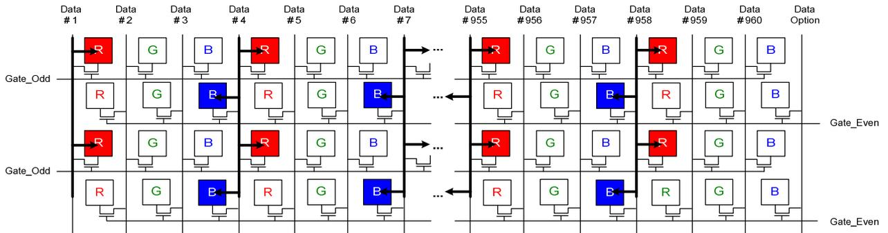
The below figure is Z-inversion panel driving method. The panel will be drive by the Red data input of the Gate\_Odd and the Green data input of the Gate\_Even.
