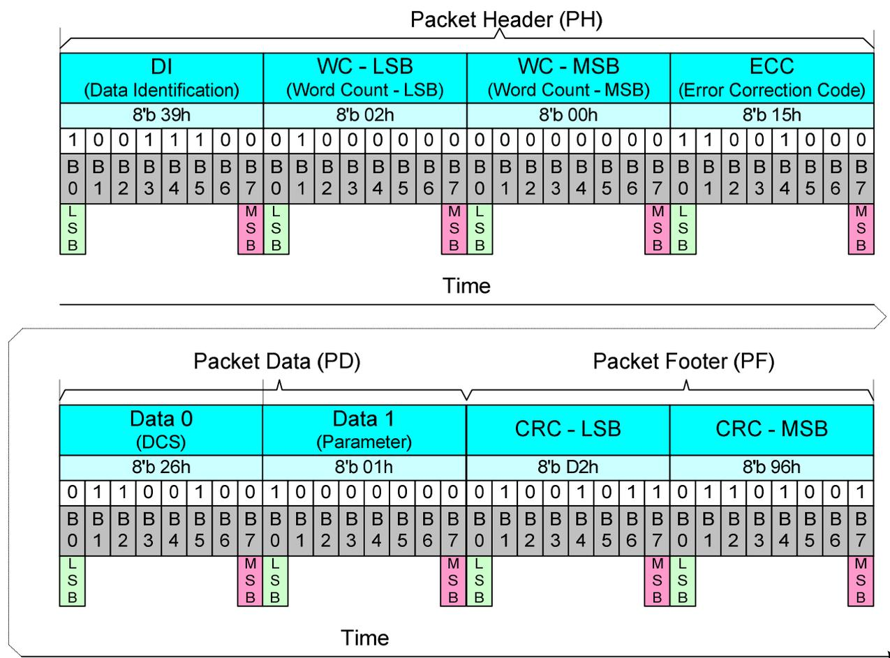
Long Packet (LPa), when a Write (4 parameters) was sent, is defined e.g.
