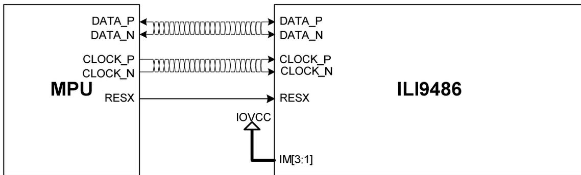
Low Power mode means that each line of the differential pair is used in single end mode and a differential receiver is disabled (A termination resistor of the receiver is disabled) and it can be driven into a low power mode. High Speed mode means that differential pairs (The termination resistor of the receiver is enabled) are not used in the single end mode.
