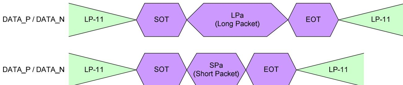
The multiple packets in High-Speed Data Transmission is illustrated for reference purposes below:
