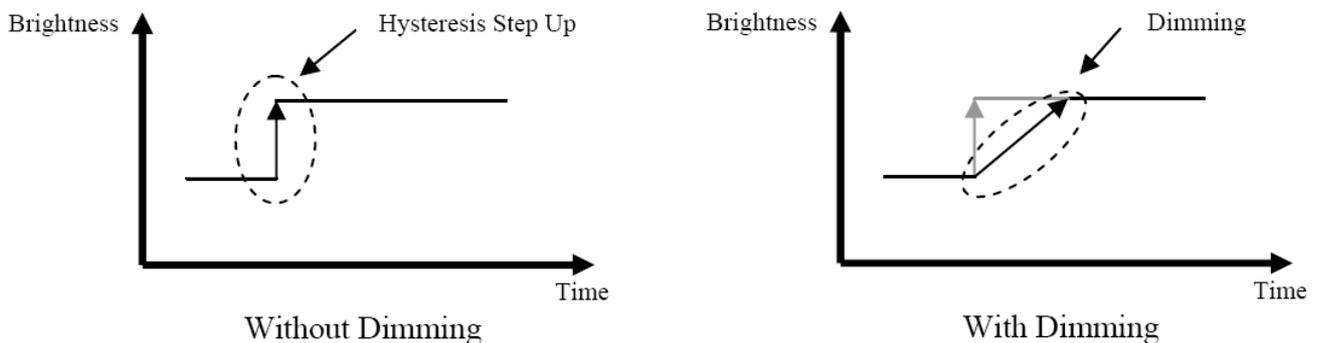
Dimming function can be enabled and disabled. See command "Write CTRL Display(53h), bit3(DD) for more information.
