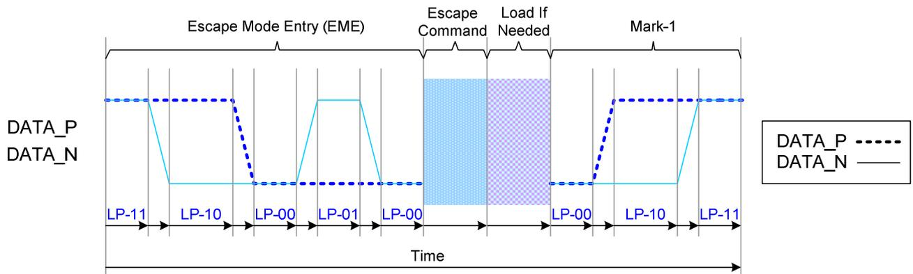
Note: Load (Data) is presenting that the first bit is logical '1' in this example.
