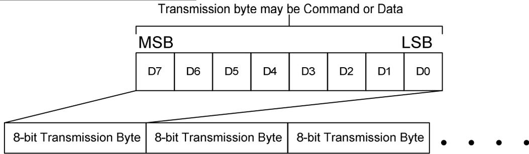
The host drives the CSX pin to low and starts by setting the D/CX bit on SDA. The bit is read by ILI9486 on the first rising edge of SCL signal. On the next falling edge of SCL, the MSB data bit (D7) is set on SDA by the host. On the next falling edge of SCL the next bit (D6) is set on SDA. If the optional D/CX signal is used, a byte is eight read cycle long. The 3/4-line serial interface writes sequence described in the Figure as below.
