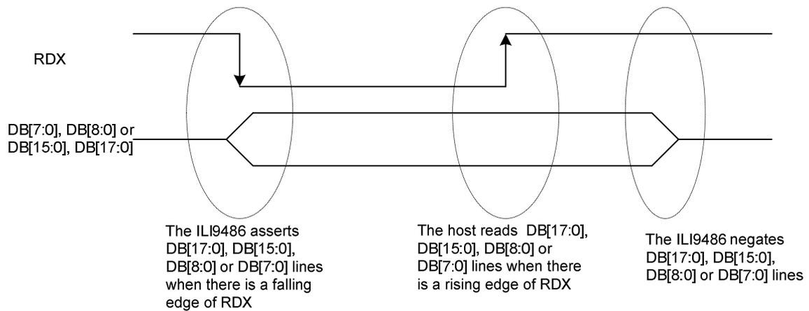
Note: RDX is an unsynchronized signal (It can be stopped).
