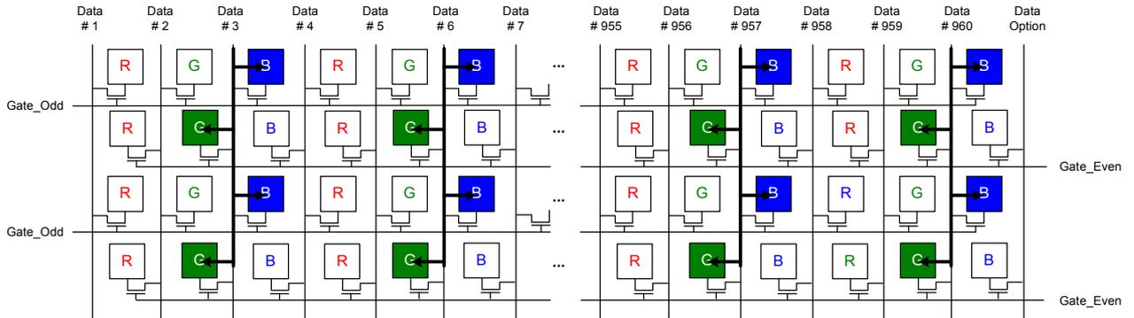
The below figure is Z-inversion panel driving method. The panel will be drive by the Blue data input of the Gate\_Odd and the Red data input of the Gate\_Even.
