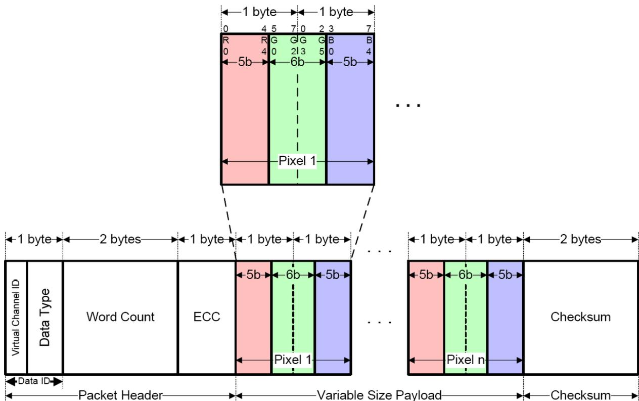
**7.7.10. MIPI – 18-bit per Pixel, Long packet, Data Type = 01 1110 (1Eh)**
