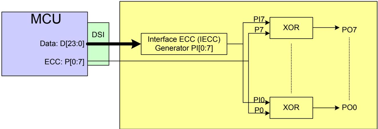
The sent data bits (D[23...0]) and ECC (P[7...0]) are received correctly, if a value of the PO[7...0] is 00h.
