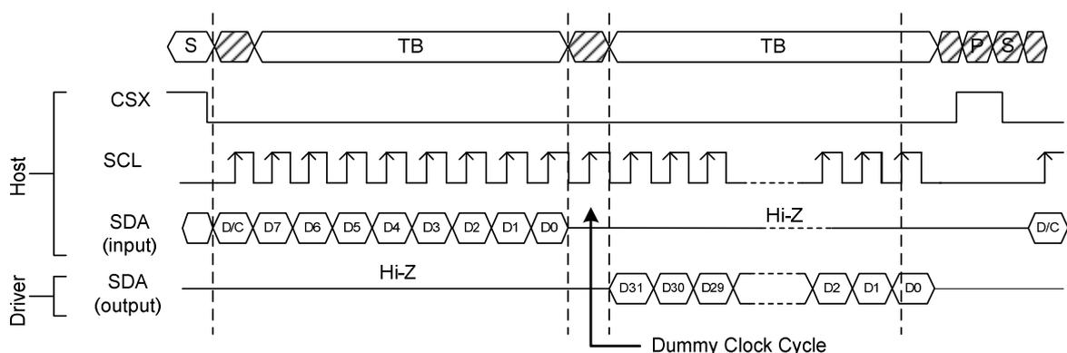
4-line Serial Protocol (for RDID1/RDID2/RDID3/0Ah/0Bh/0Ch/0Dh/0Eh/0Fh command: 8-bit read)
