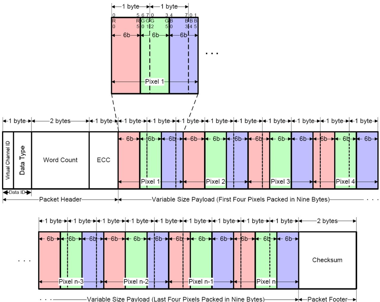
**7.7.11. MIPI – 18-bit per Pixel, Long packet, Data Type = 10 1110 (2Eh)**
