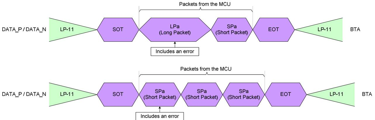
Therefore, there is needed a method to check if there has been errors on the previous packets. These errors of the previous packets can check “Read Display Signal Mode (0Eh)” and “Read Number of the Errors on DSI (05h)” commands.
