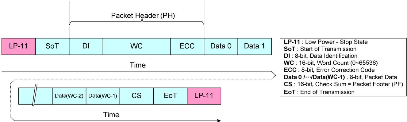
The other possibility is that there is not needed SoT, EoT and LP-11 between packets if packets have sent in multiple packet format e.g.
