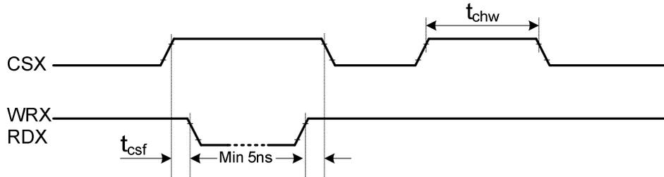
(3) Logic high and low levels are specified as 30% and 70% of IOVCC for input signals.
