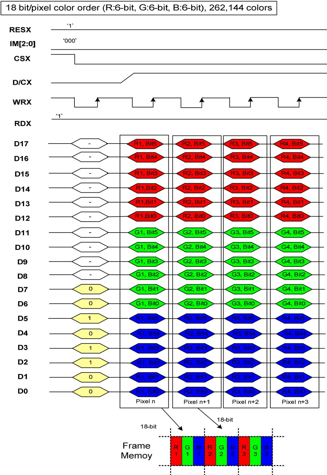
Note 1: The data order is as follows, MSB=D17, LSB=D0 and picture data is MSB=Bit 5, LSB=Bit 0 for Green and MSB=Bit4, LSB=Bit0 for Red and Blue data.
