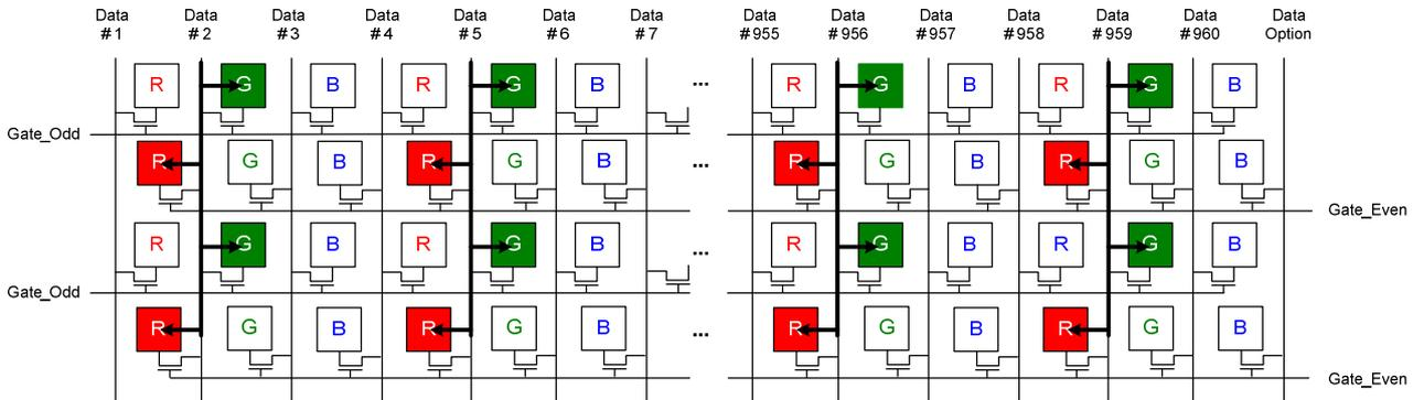
The below figure is Z-inversion panel driving method. The panel will be drive by the Green data input of the Gate\_Odd and the Blue data input of the Gate\_Even.
