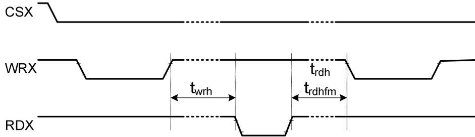
**17.3.2. Display Serial Interface Timing Characteristics (3-line SPI system)**
