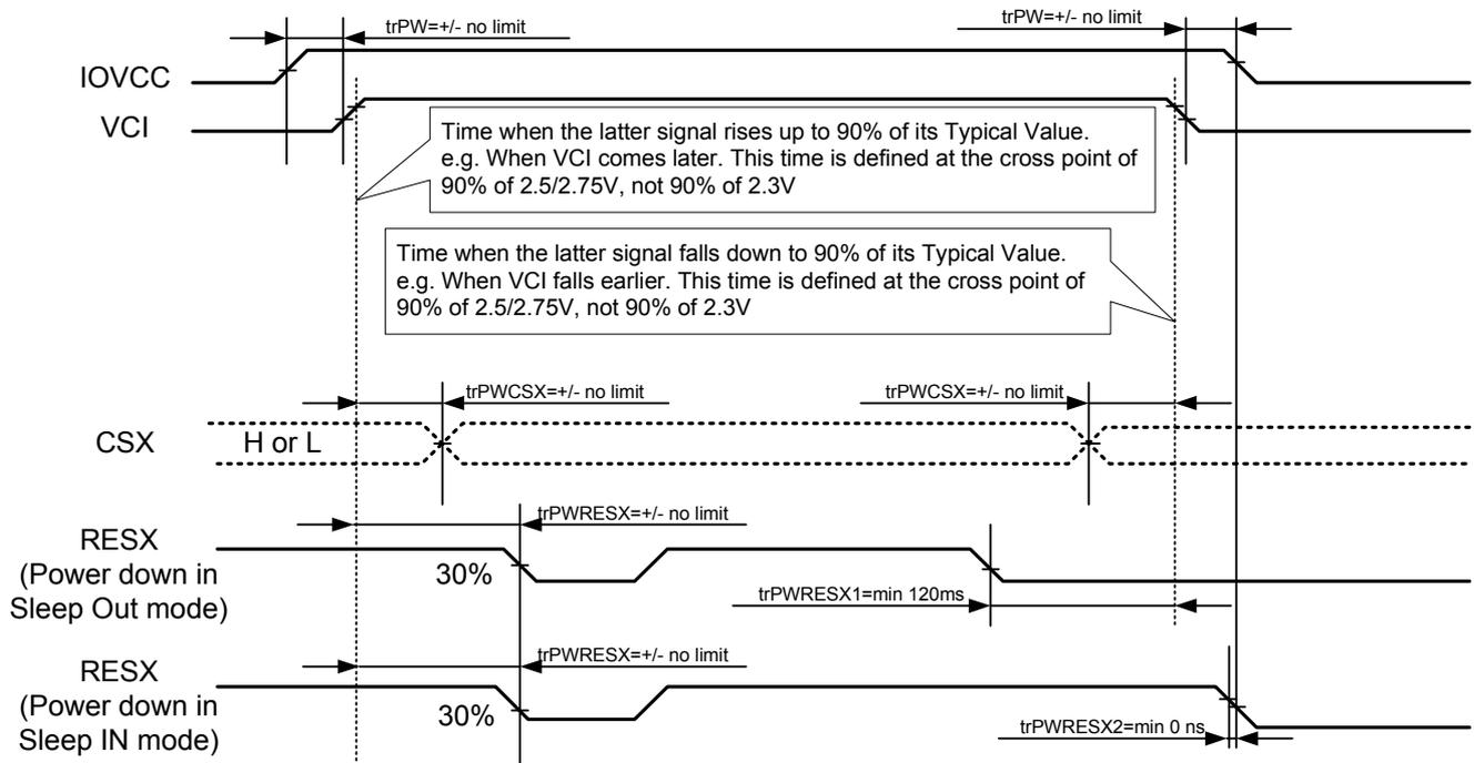
trPWRESX1 is applied to RESX falling in the Sleep Out Mode
