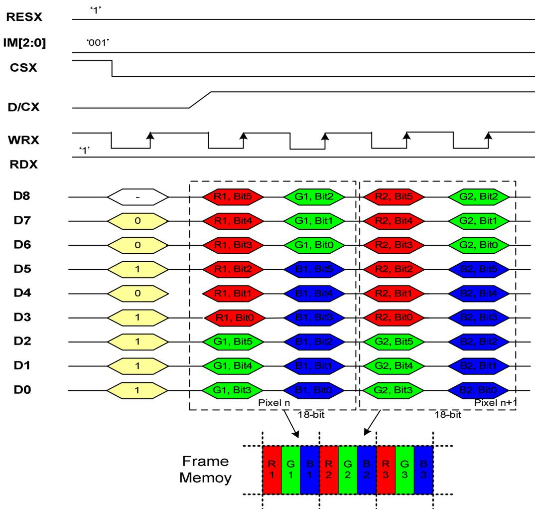
Note 1: The data order is as follows, MSB=D8, LSB=D0 and picture data is MSB=Bit 5, LSB=Bit 0 for Green, Red and Blue data.
