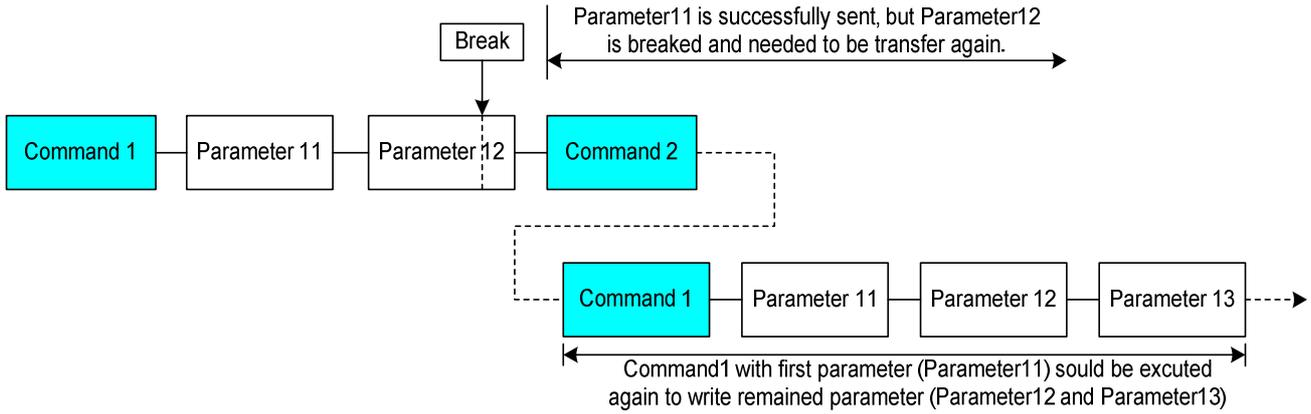
If a two or more parameter command is being sent and a break occurs by the other command before the last one is sent, then the parameters that were successfully sent are stored and the other parameter of that command remains previous value.
