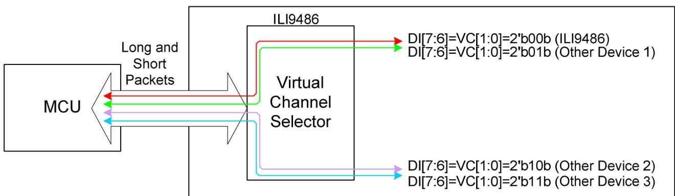
Virtual Channel (VC) is always 0 ( $DI[7..6]=VC[1..0]=00b$ ) when the MCU is sending "End of Transmission Packet" to the display module.
