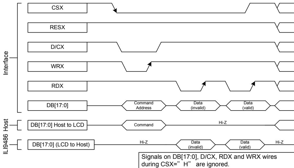
Note: Read Data is only valid when the D/CX input is pulled high. If D/CX is driven low during read then the display information outputs will be High-Z.
