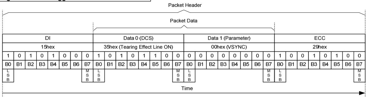
**Tearing Effect Bus Trigger Enable - Long Packet**
