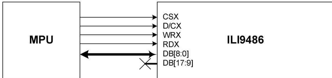
18 bit/pixel color order (R:6-bit, G:6-bit, B:6-bit), 262,144 colors
