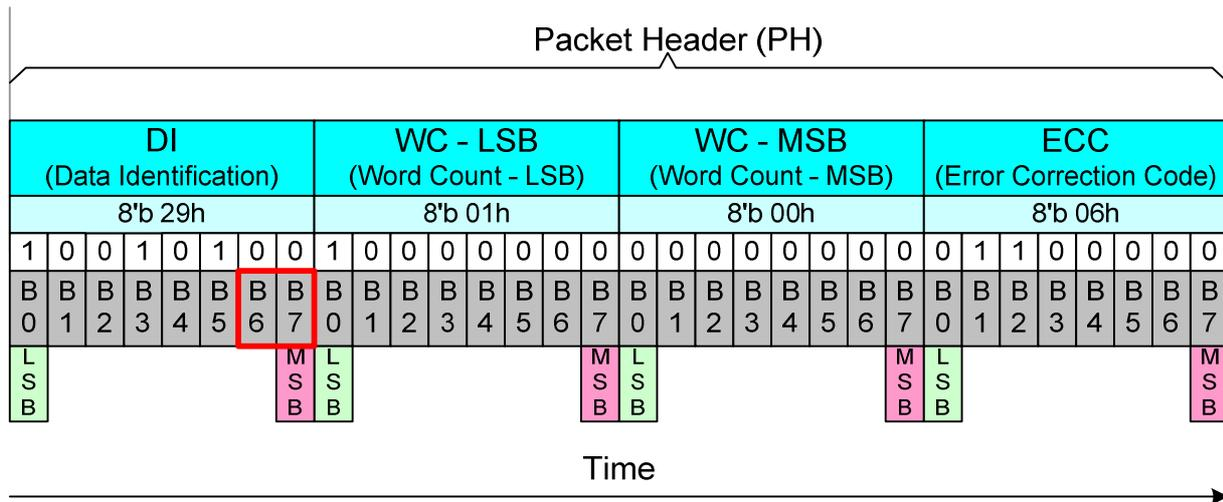
Virtual Channel (VC) can address 4 different channels for e.g. 4 different display modules. Devices are using the same virtual channel what the MCU is using to send packets to them e.g.
