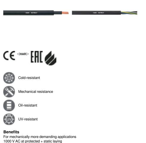
Arrangements made of single-core, rubber-sheathed cables H07RN-F can be used for short circuit-proof and short-to-ground-proof installations in accordance with IEC 60364-5-52/ HD 60364-5-52/ VDE 0100 Part 520
