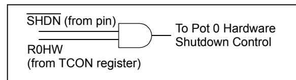
**FIGURE 5-12:** R0HW bit and  $\overline{\text{SHDN}}$  pin Interaction.
