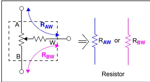
FIGURE 5-8: Rheostat Configuration.
