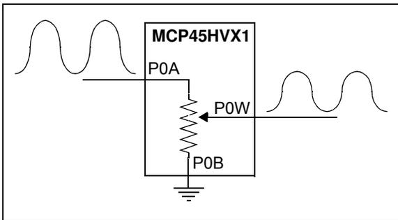
**FIGURE 8-10:** Signal Attenuation Block Diagram – Ground Referenced.
