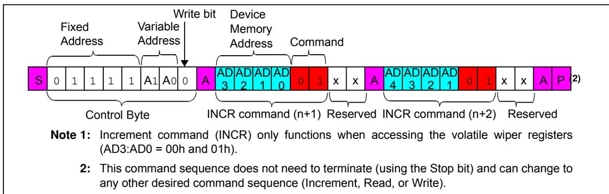
**FIGURE 7-7:** I<sup>2</sup>C Increment Command Sequence.
