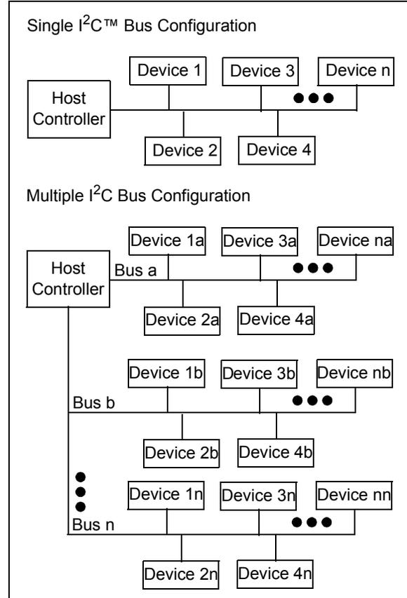
**FIGURE 8-11:** Typical Application I<sup>2</sup>C Bus Configurations.
