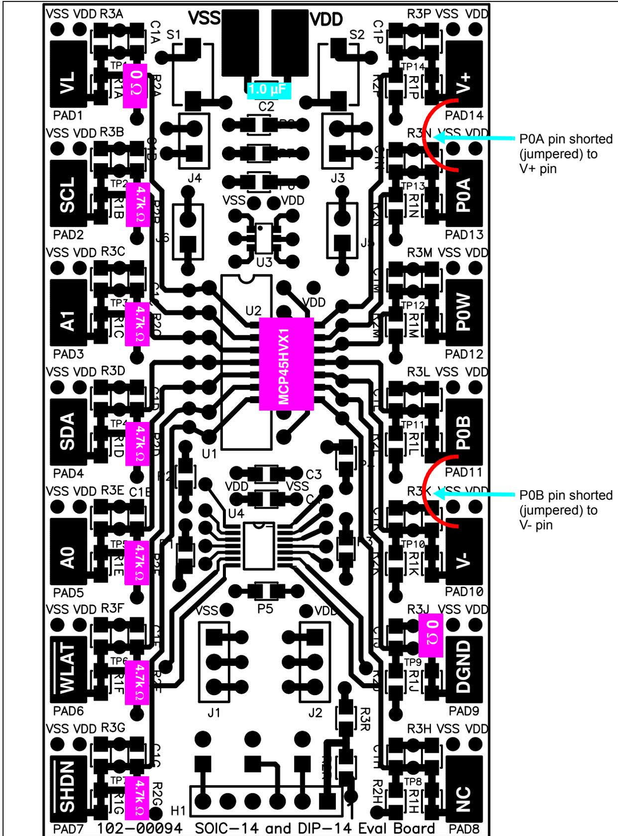
FIGURE 10-2: Digital Potentiometer Evaluation Board Circuit Using SOIC14EV.
