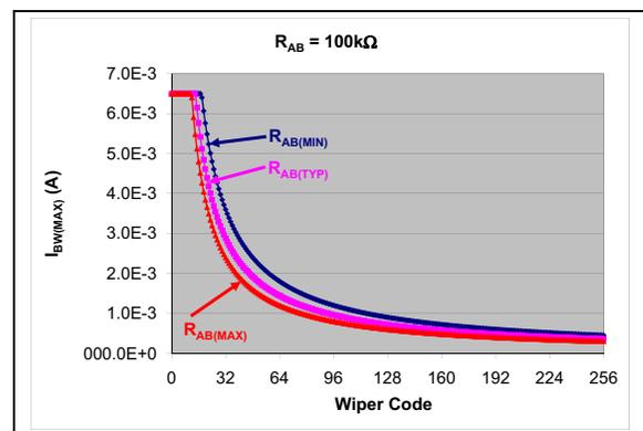
**FIGURE 5-6:** Maximum  $I_{BW}$  vs Wiper Code - 100 kΩ .
