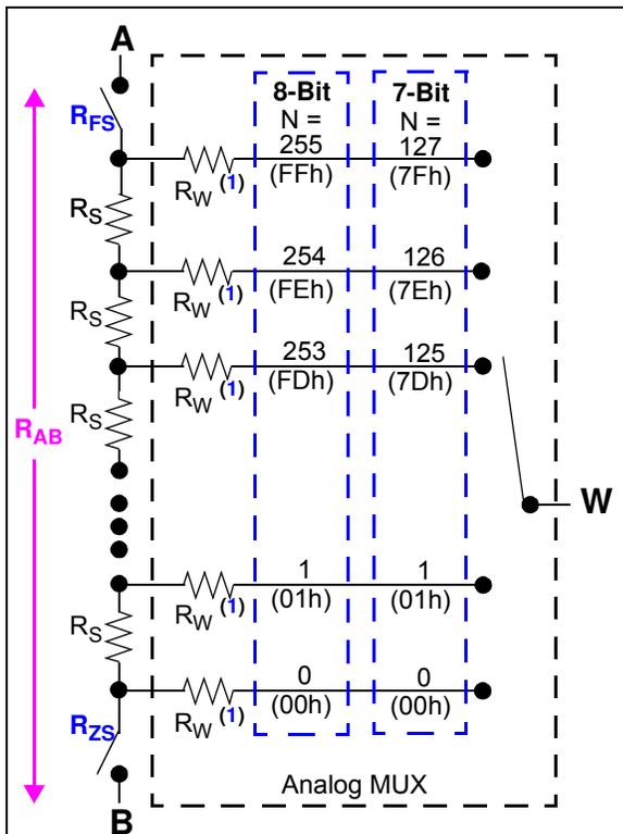
**Note 1:** The wiper resistance is dependent on several factors including wiper code, device V+ voltage, terminal voltages (on A, B and W), and temperature. Also for the same conditions, each tap selection resistance has a small variation. This R<sub>W</sub> variation has greater effect on some specifications (such as INL) for the smaller resistance devices (5.0 kΩ) compared to larger resistance devices (100.0 kΩ).
