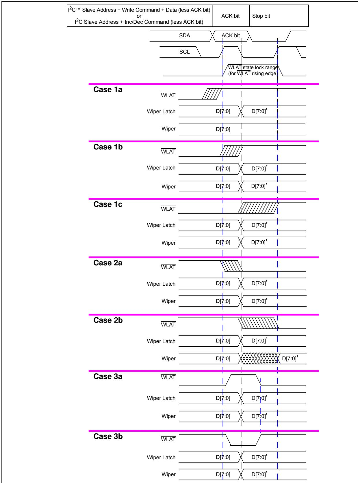
**FIGURE 4-7:**  $\overline{\text{WLAT}}$  Interaction with I<sup>2</sup>C ACK Pulse
