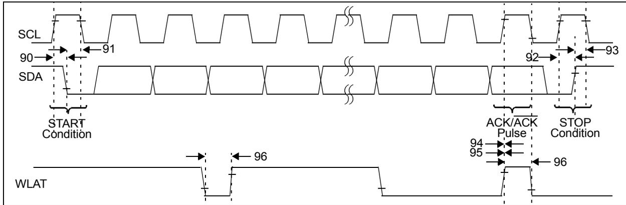
**FIGURE 1-2:** I<sup>2</sup>C Bus Start/Stop Bits Timing Waveforms.
