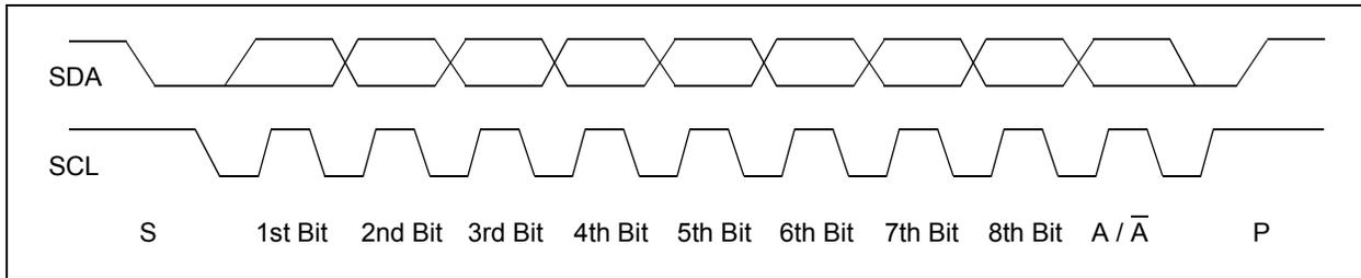
**FIGURE 6-7:** Typical 8-Bit I<sup>2</sup>C Waveform Format.
