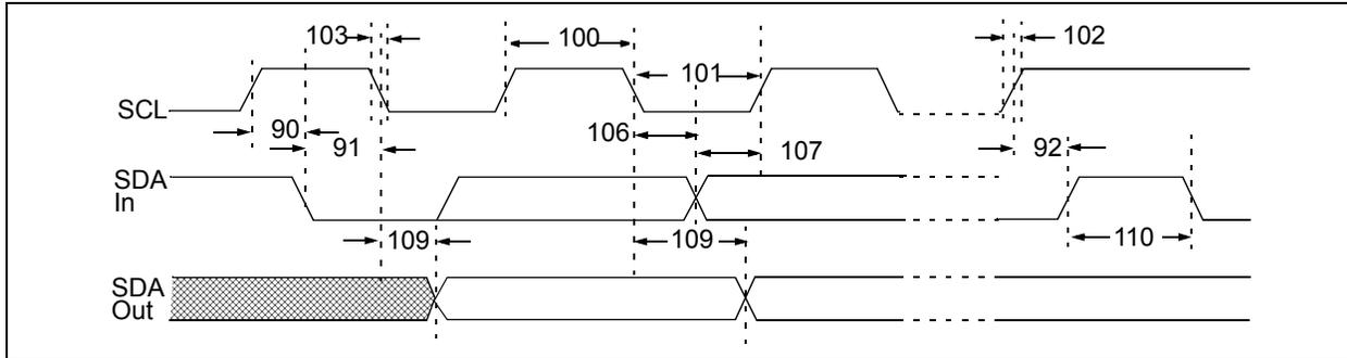
FIGURE 1-3: I<sup>2</sup>C Bus Timing Waveforms.
