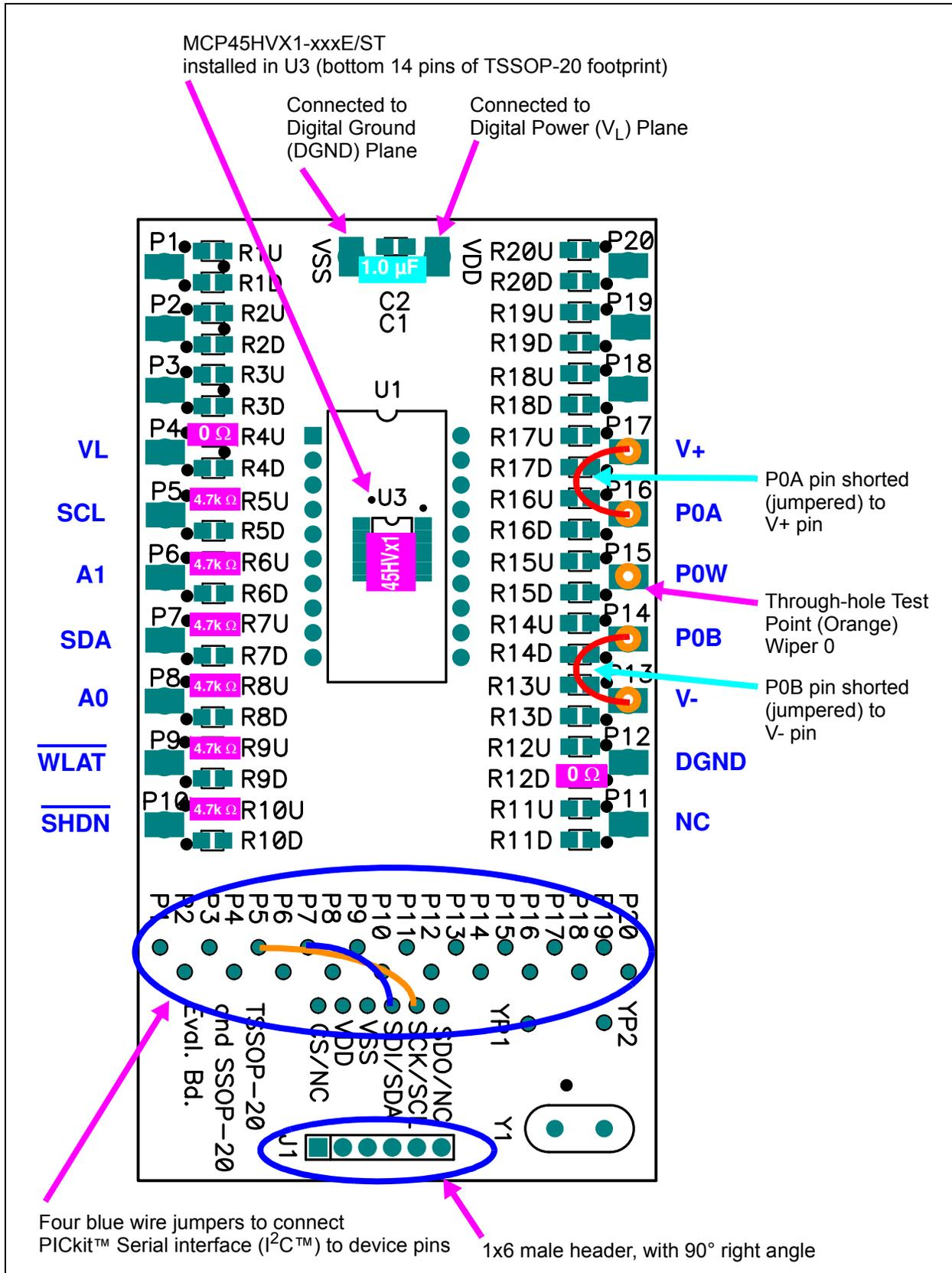
**FIGURE 10-1:** Digital Potentiometer Evaluation Board Circuit Using TSSOP20EV.
