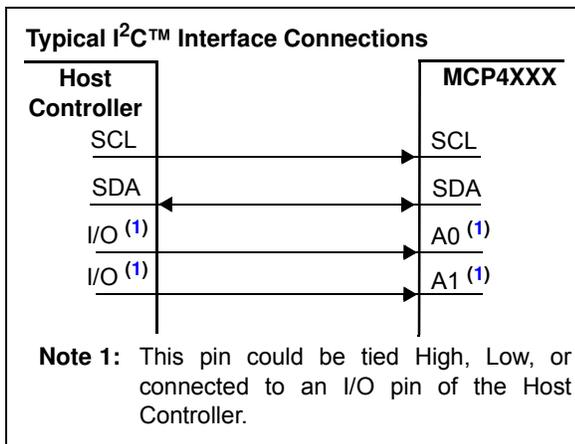
**FIGURE 6-1:** Typical I<sup>2</sup>C Interface Block Diagram.
