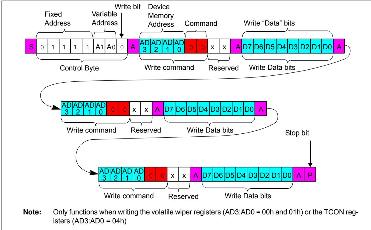
**FIGURE 7-3:** I<sup>2</sup>C Continuous Volatile Wiper Write.
