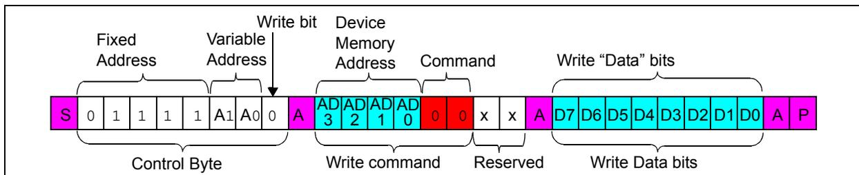
**FIGURE 7-2:** I<sup>2</sup>C Write Sequence.
