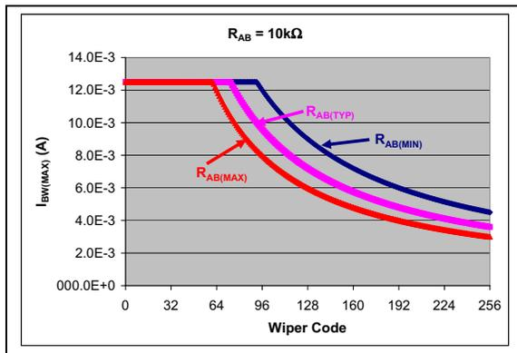
**FIGURE 5-4:** Maximum  $I_{BW}$  vs Wiper Code - 10 kΩ .
