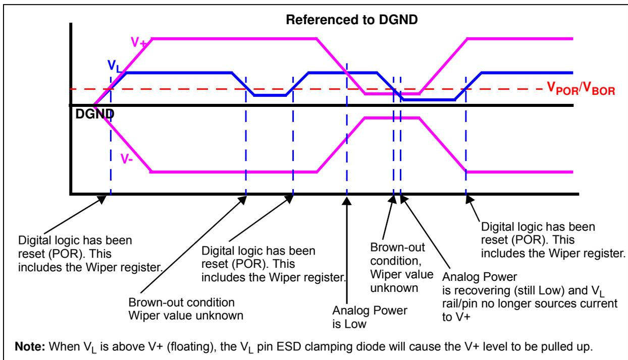
**FIGURE 4-3:** DGND, V<sub>L</sub>, V+, and V- Signal Waveform Examples.
