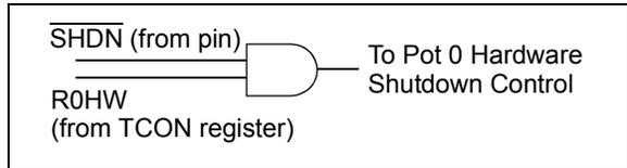
**FIGURE 4-6:** R0HW bit and  $\overline{\text{SHDN}}$  pin Interaction.
