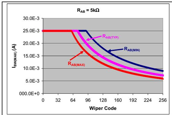
**FIGURE 5-3:** Maximum  $I_{BW}$  vs Wiper Code - 5 kΩ .
