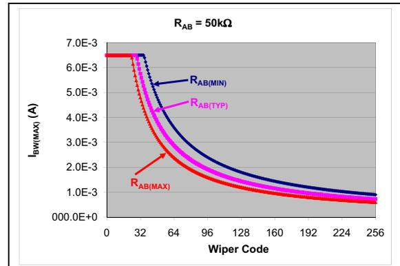
**FIGURE 5-5:** Maximum  $I_{BW}$  vs Wiper Code - 50 kΩ .
