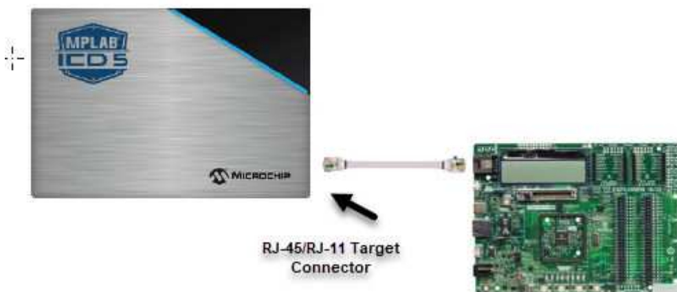
Figure 3-5. MPLAB ICD 5 Unit to Target Connection
