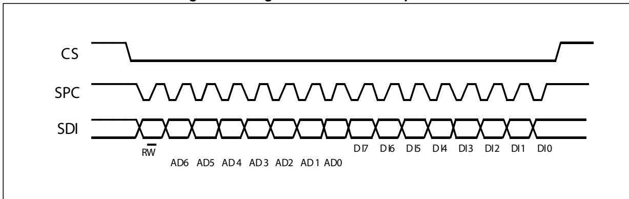
The SPI write command is performed with 16 clock pulses. The multiple byte write command is performed by adding blocks of 8 clock pulses to the previous one.
