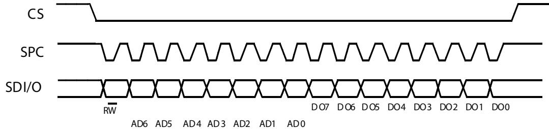
The SPI read command is performed with 16 clock pulses:
